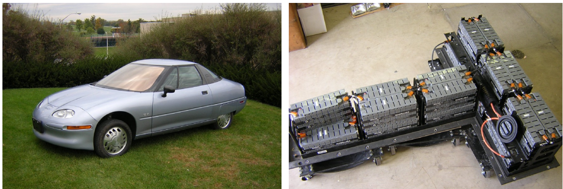
Figure 1.2: Penn State HyLion vehicle and battery pack
