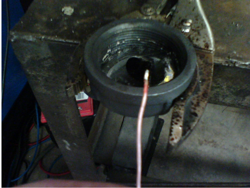
Figure 3.28: Tinning the litz wire
