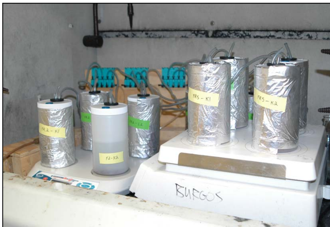
Figure 4-3: Picture of batch reactors in a laboratory fume hood. The third stir plate is located in the back right of the hood. The gas mix is fed through a main line on the left to the three teal-colored aquarium manifolds and then to the reactors. Aluminum foil was removed from one of the reactors for illustration purposes.
