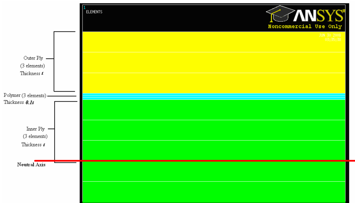
Figure 3-16: Close-up of Meshed Layers in ANSYS Model
