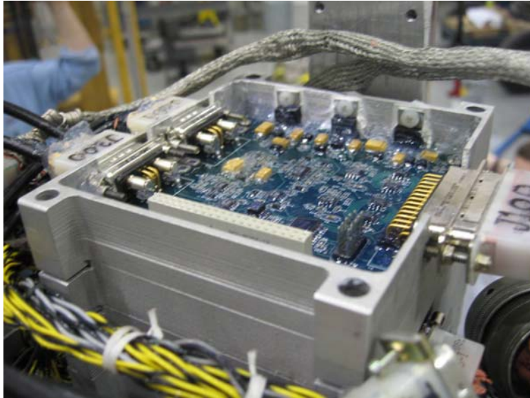
Figure 4.32 - Photograph of the power and processing board for ESPRIT. Note the mounting of the linear regulators to the box.
