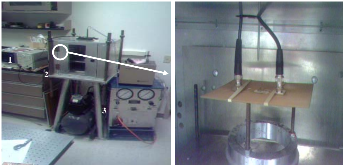
Figure 4.9. (a) Experimental setup for monitoring the localized changes in mechanical behavior of a polymer film including 1. Network Analyzer, 2. Oven, and 3. Thermocouple controller along with (b) a close up image of the device under test showing the BNC connections and the thermocouple used for temperature monitoring.
