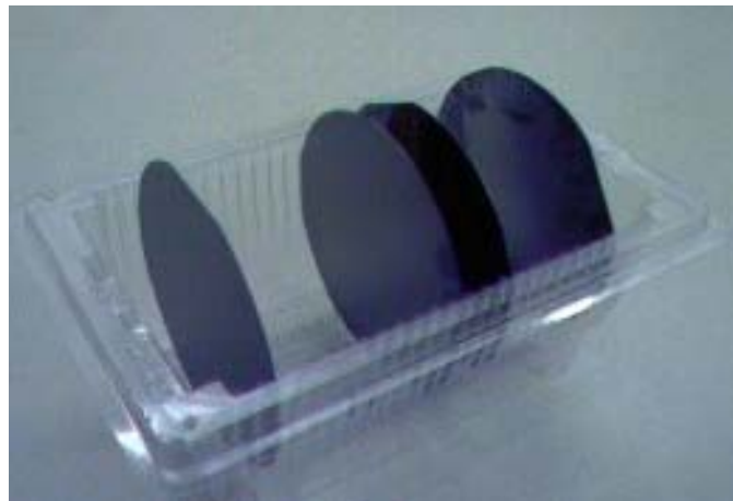
Figure 5.6. Photograph of the 3" diameter silicon wafers coated with SU-8 films for the Nanoindentation tests comparing exposed and unexposed films.
