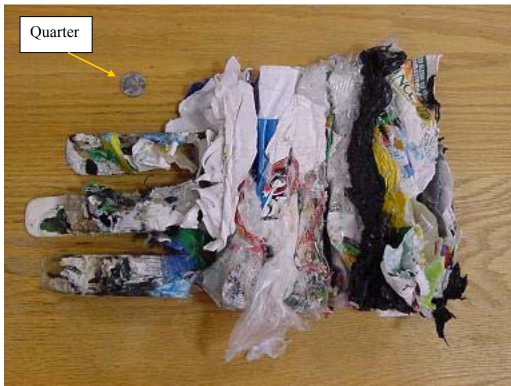
Figure 34: Plug Removed from Machine During Initial Testing
