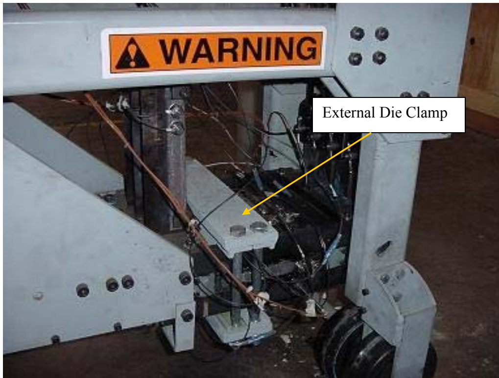
Figure 41: Die Assembly with External Clamp
