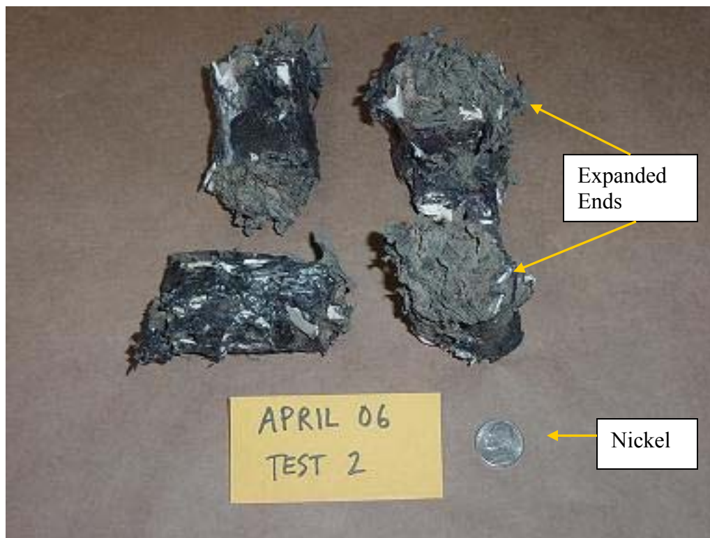
Figure 52: Four Nuggets Produced with Die Temperature of 220°C
