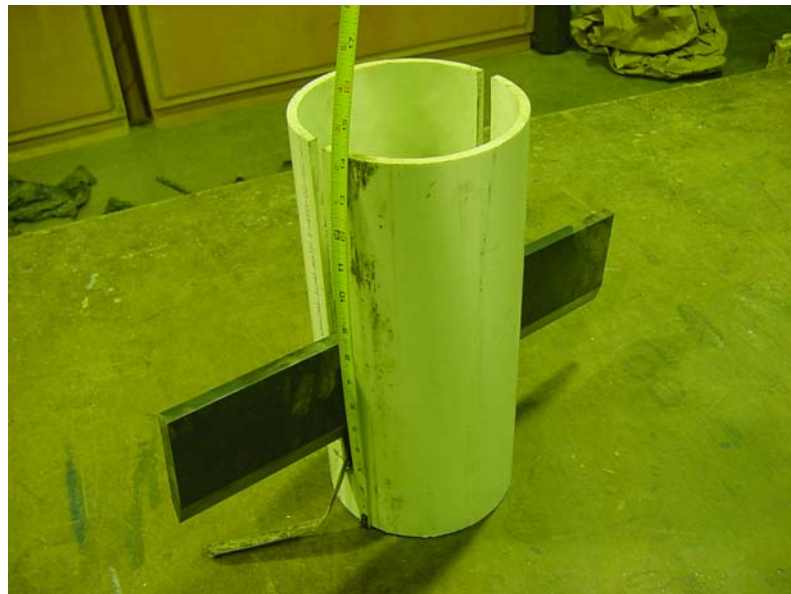
Figure 6: PVC Tube Used for Density at Cutting and Knife Temperature Relationship
