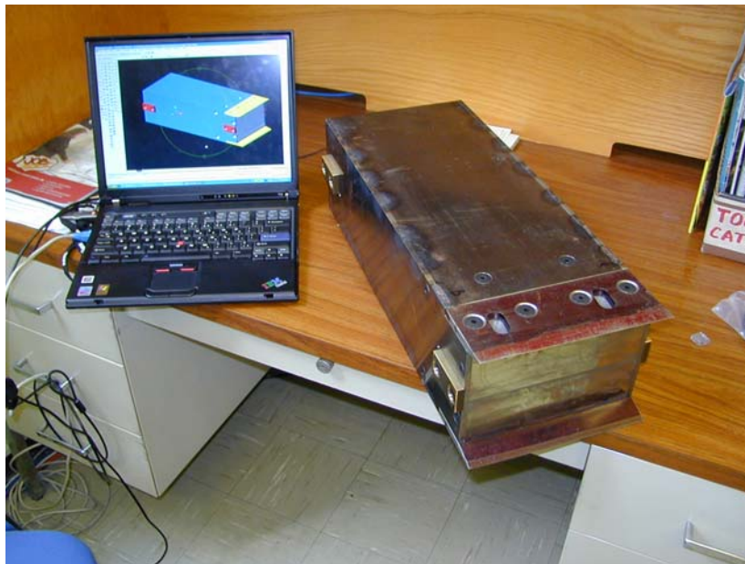
Figure 22: Compaction Plunger and CAD Drawing
