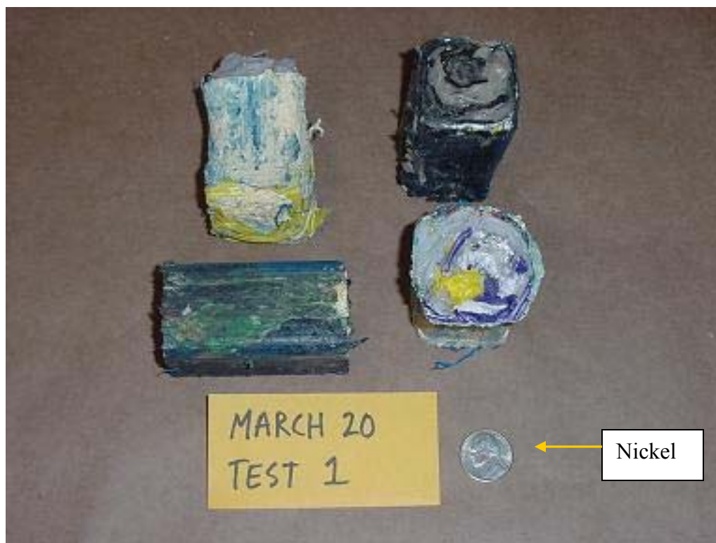
Figure 54: Four Nuggets Produced with Die Temperature of 125°C
