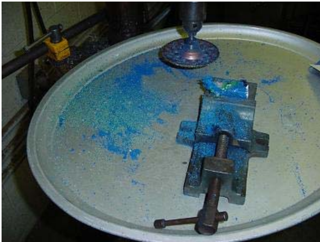
Figure 33: Plastofuel™ Sample Preparation for Calorimetry Testing
