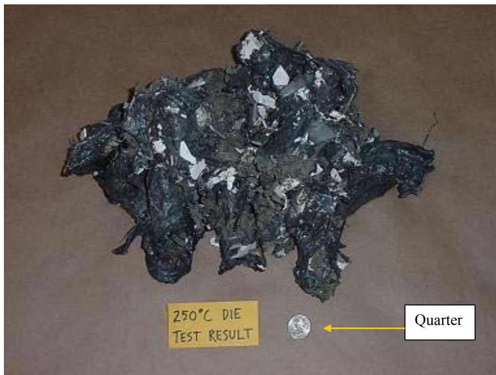
Figure 51: 250°C Test Result - Solid Mass of Melted and Unmelted Plastic
