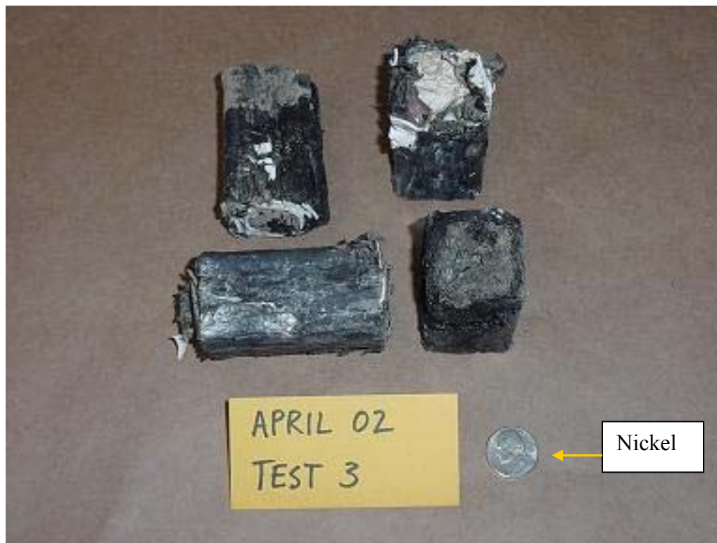
Figure 55: Four Nuggets Produced with Die Temperature of 155°C
