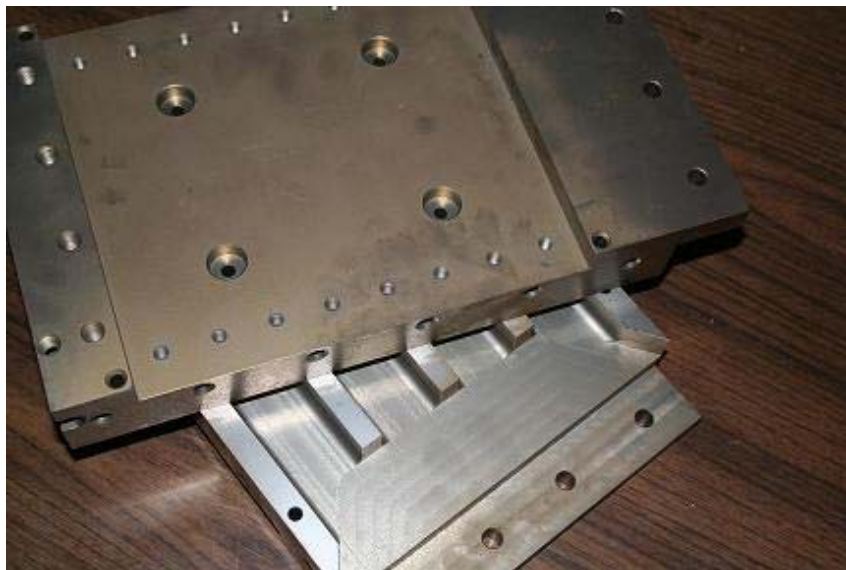
Figure 25: Die Halves Prior to Assembly
