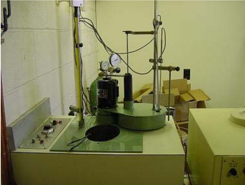
Figure 32: Bomb Calorimeter Used for Plastofuel™ Energy Content Analysis
