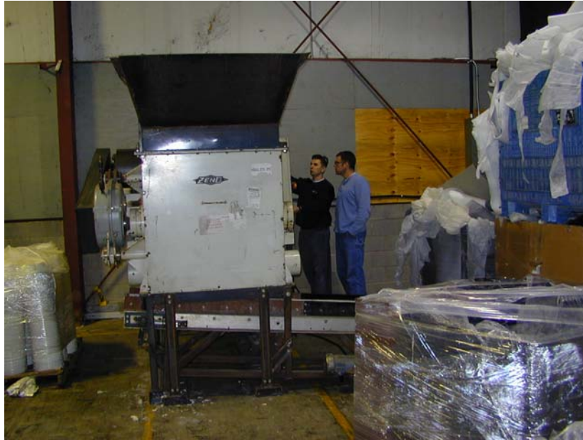
Figure 38: Zeno ZTL 1000x1200 Shredder Used to Shred Plastic Film and Rigid
