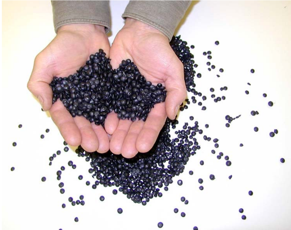
Figure 4: Plastic Fuel Pellets for GR Technologies Burner
