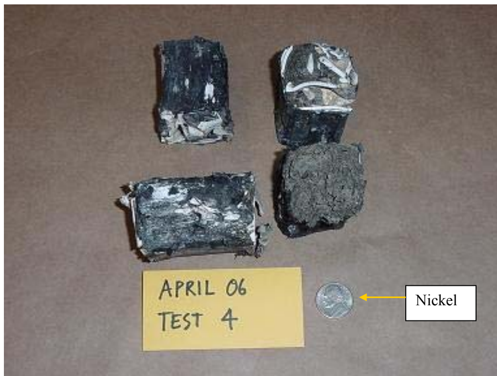
Figure 56: Four Nuggets Produced with Die Temperature of 175°C
