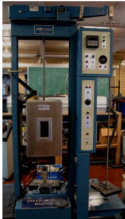
Figure 6.22: Creep frame used for the creep test at PSU.
