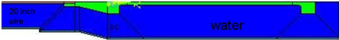
Figure 6.11: Axi-symmetric geometry for a pulse-echo measurement with a transitional ‘horn.’ Time-domain finite element modeling was performed for a specimen in water (shown) and for a specimen in air (not shown).
