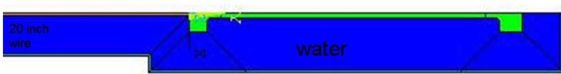
Figure 6.9: Axi-symmetric geometry for a pulse-echo measurement without using transitional ‘horns.’ Time-domain finite element modeling was performed for a specimen in water (shown) and for a specimen in air (not shown).
