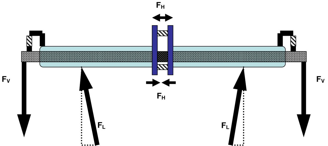
**Figure A.2.** A representative free body diagram of the bar and the forces acting on and across it.  $F_L$  is the force applied by the lifter (one for each arm),  $F_V$  is the force of the bar and the weights loaded onto each end, and  $F_H$  is the horizontal force acting along the long axis of the bar.
