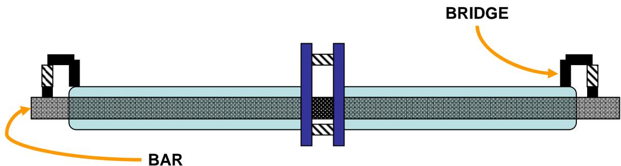
**Figure A.1.** A schematic of the instrumented bar designed for this study. The two vertical plates are connected via three horizontally-mounted force transducers. The grip portion of the regular bar runs through the two sleeves and is suspended in place by a vertically-mounted force transducer at each end. A small “bridge” was built that extended up and past the end of the sleeve so that the transducer could be mounted in a straight, vertical line. The figure is not to scale.
