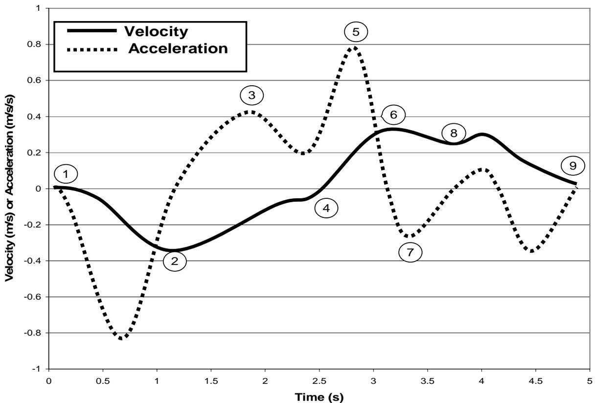
**Figure 2.1:** Typical vertical bar velocity and acceleration during the bench press. The nine point markers coincide with those described by Madsen and McLaughlin (1984) and discussed in the text.
