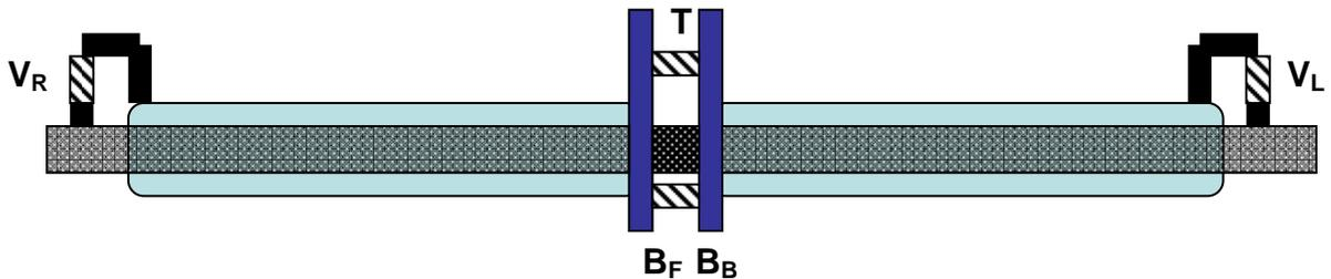
**Figure A.3.** Illustration of the locations of the various transducers. In this view the two bottom transducers are located immediately in front and back of each other. While the illustration is not to scale, the distance from the center of the bar to  $T$  was double that of vertical distance to  $B_F$  and  $B_B$ .
