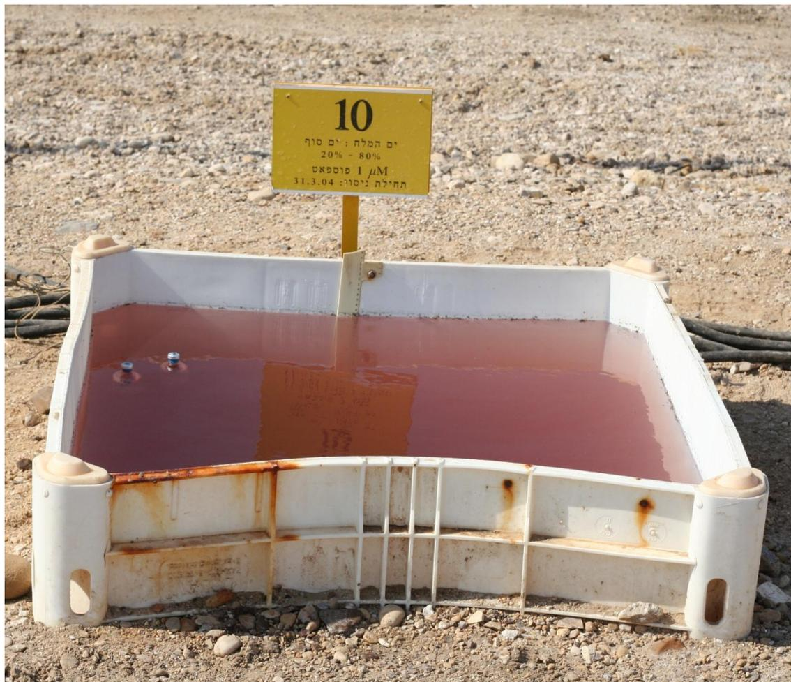
**Figure 1-4.** Photograph depicting a close up of one of the Dead Sea research pools located at the Dead Sea Works facility, Sdom, Israel (07/22/2007). This pool, Pool 10, contains approximately 1 m<sup>3</sup> of water of which 80% is from the Dead Sea (salinity ≈350‰) and 20% is from the Red Sea (salinity ≈41‰). The pool was fertilized with 1 μM phosphate to promote microbial growth. The red color of the pool is due to the carotenoids present in the membranes of member of the Haloarchaea.
