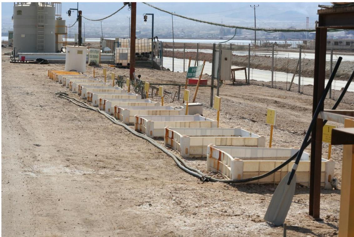
**Figure 1-3.** Photograph depicting the installation of Dead Sea research pools located at the Dead Sea Works facility, Sdom, Israel (07/22/2007). Each pool contains approximately  $1 \text{ m}^3$  of water of various mixtures of Dead Sea and Red Sea waters.
