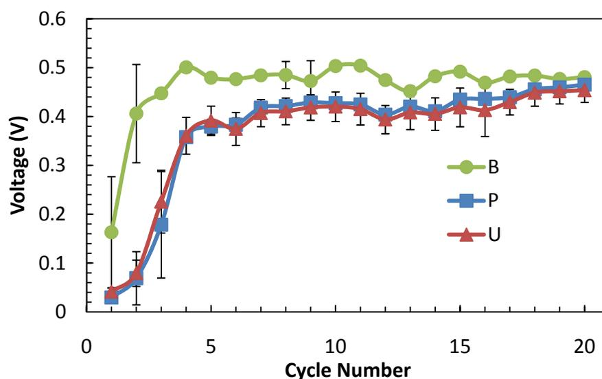
Figure 3.1. Plot of average maximum voltage for each cycle. Initially Bog-inoculated reactors (B) produce more voltage than wastewater inoculated reactors (P, PSU) (U, UAJA). By day 60 all reactors produce similar voltages. Wastewater reactors produce the similar voltages throughout the length of the experiment.
