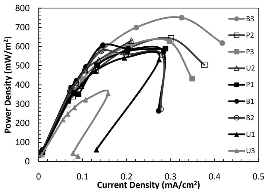
Figure 3.2. Power density curves generated from cycle 16 (day 48) showing that UAJA replicate 3 produced significantly ( $t$ -test,  $\alpha = 0.05$ ,  $P = 0.005$ ) less power than all other reactors, including other UAJA replicates.
