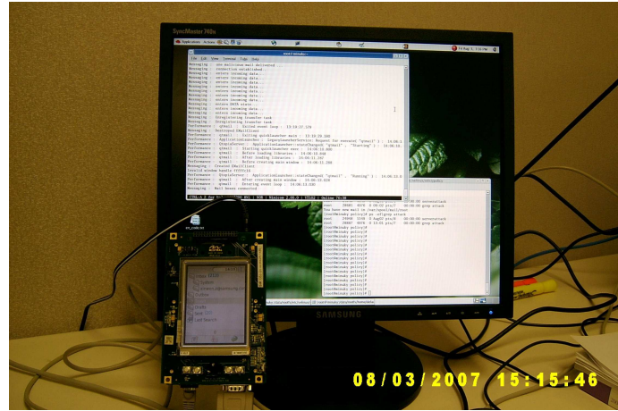
Figure 5.7. OMAP-5912OSK as a generic development platform for both WinCE and Linux-based smartphones; in our experiments, we use Linux kernel 2.6.20.4, Qtopia Phone Edition 4.2
