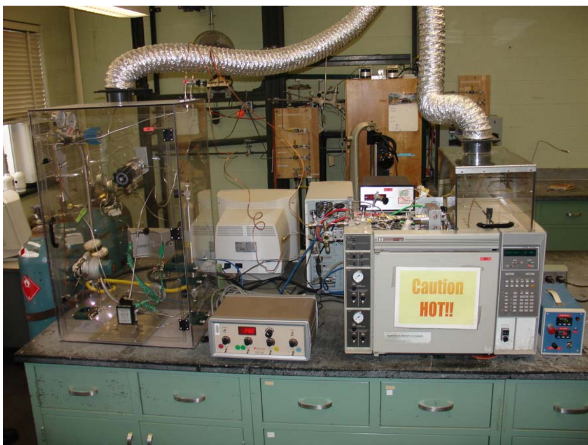
Figure 3-2: Photo of the apparatus. The gas delivery system is on the left. The HP 5890 GC appears on the right side with the injector temperature zone controller to the far right of the photo. The Tylan mass flow controller interface sits between the GC and gas delivery system. Overhead vents are used to remove exhaust gases generated during experimentation.
