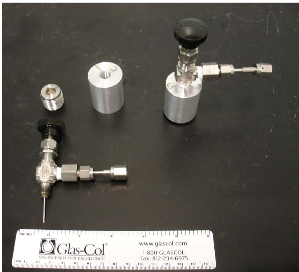
Figure 4-2: Photo of capsule body. In the upper right-hand corner is a full assembled capsule. At top left, is the plug which fits into the bottom of the capsule body (upper middle of photo). At bottom left is a picture of the valve assembly with attached needle port.
