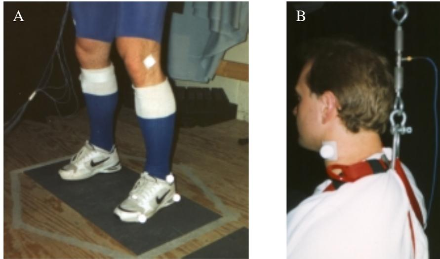
**Figure 3.2. Bertec force plate (A) and axial force transducer (B).**
