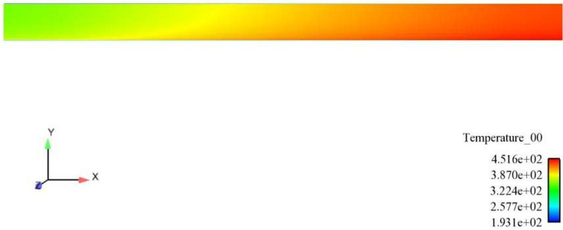
**Figure 0.6: Predicted Contours of Liquid Temperature on Clean Surface ( $q'' = 2000$  kW/m<sup>2</sup>)**
