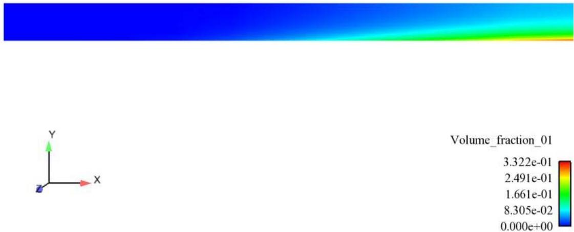
**Figure 4.14: Predicted Contours of Vapor Volume Fraction on Clean Surface ( $q'' = 2000$  kW/m<sup>2</sup>)**
