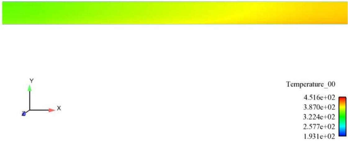
**Figure 0.8: Predicted Contours of Liquid Temperature on Clean Surface ( $q'' = 900 \text{ kW/m}^2$ )**
