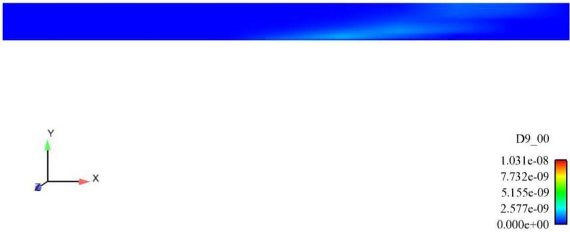
**Figure 4.20: Predicted Contours of Condensation Mass Transfer of Liquid on Clean Surface ( $q'' = 900 \text{ kW/m}^2$ )**
