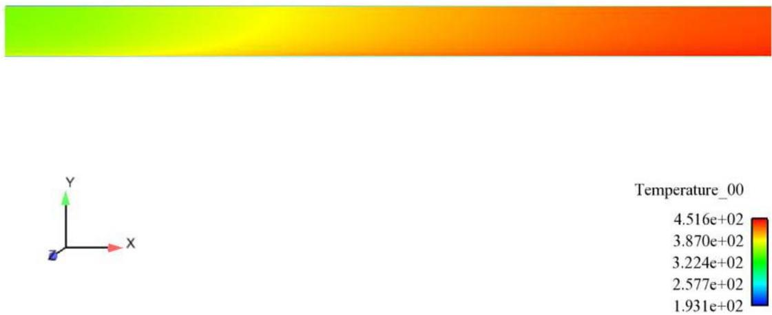
**Figure 0.7: Predicted Contours of Liquid Temperature on Crudded Surface ( $q'' = 2000$  kW/m<sup>2</sup>)**
