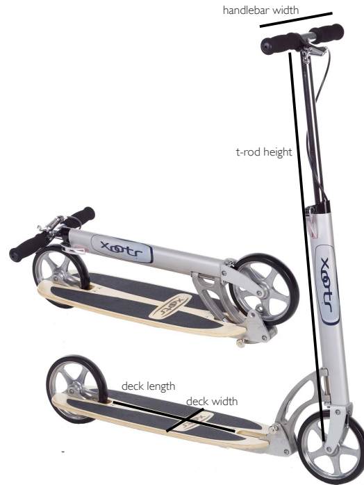
Figure 6.1: Design parameters for a scooter : deck length, deck width, T-rod height, and handlebar width. Image courtesy : www.xootr.com [3].
