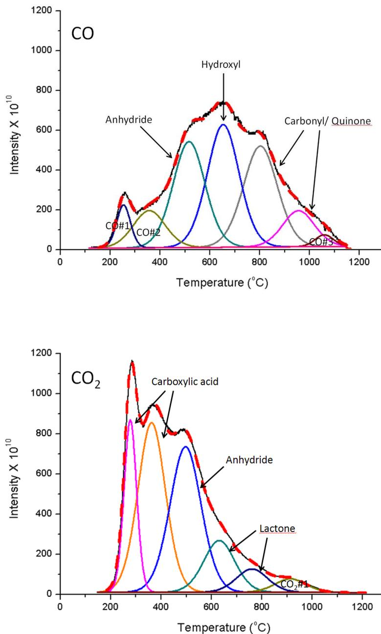
**Figure 4.15.** Results of deconvolution of TPD spectra from OAC4
