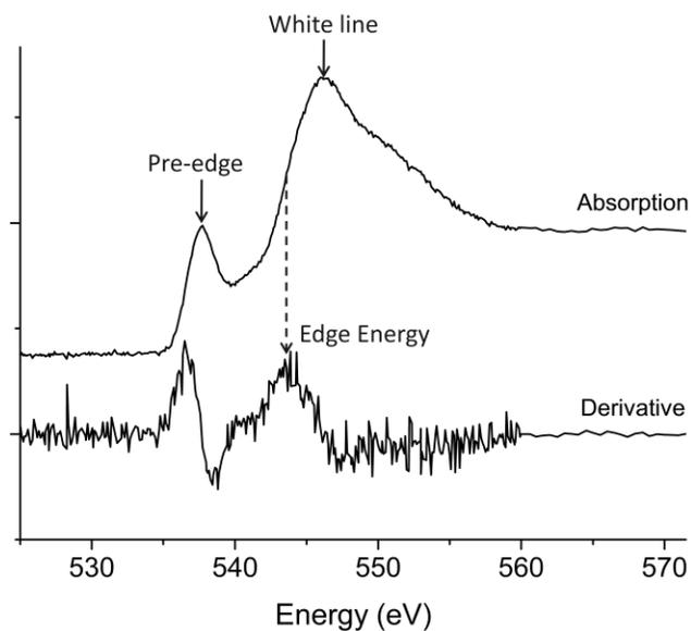
**Figure 2.5.** Oxygen K-edge XANES spectrum of an activated carbon and its first derivative
