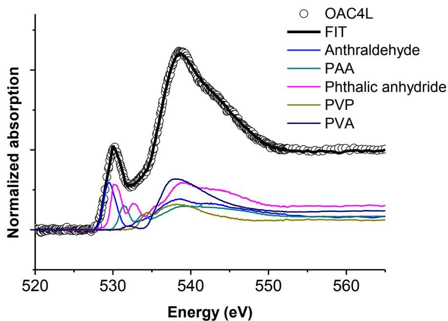
**Figure 4.13.** Fitting result of OAC4L (oxidized activated carbon treated at 250 °C)
