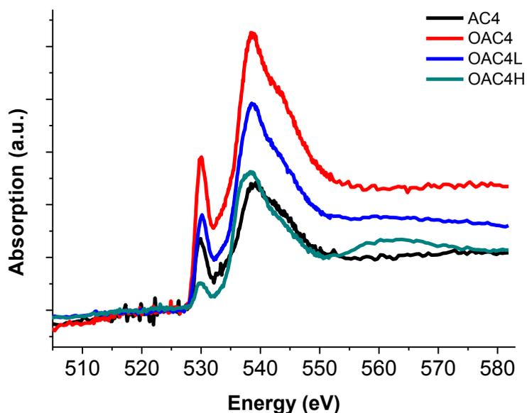
**Figure 4.10.** Oxygen K-edge XANES spectra of untreated activated carbon (AC4), oxidized activated carbon without heat treatment (OAC4), and thermally treated oxidized activated carbons at 250 °C and 1050 °C (OAC4L and OAC4H respectively)
