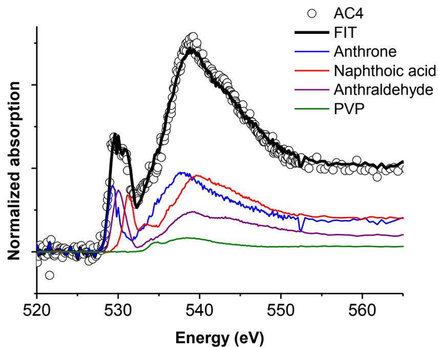
**Figure 4.11.** Fitting result of AC4 (untreated activated carbon)
