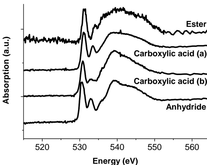
**Figure 4.6.** Oxygen K-edge XANES spectra of carboxyl-type functional groups: (1) ester (PVCVA), (2) carboxylic acid (a) (PAA), (3) carboxylic acid (b) (naphthoic acid), (4) anhydride (phthalic anhydride)
