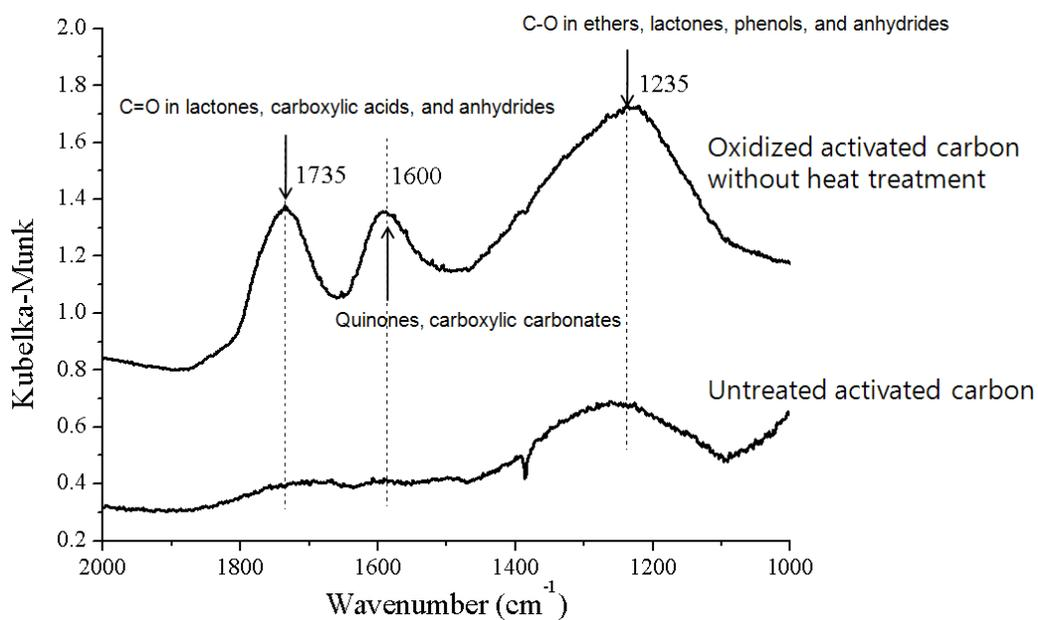
**Figure 4.18.** Peak assignments of DRIFTS results from untreated activated carbon and oxidized activated carbon without heat treatment
