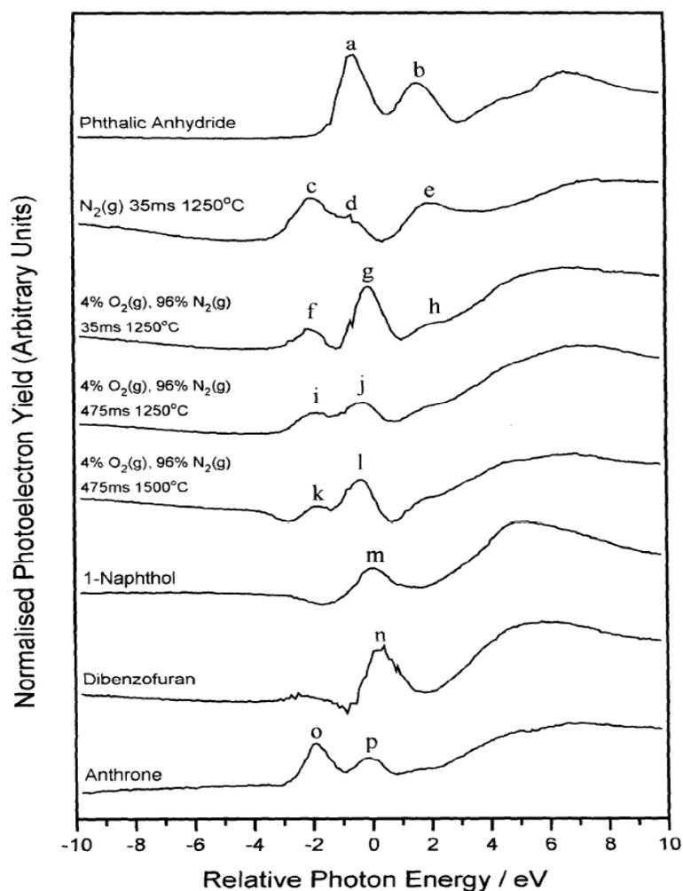
**Figure 2.6.** Oxygen K-edge XANES spectra of char samples combusted at different conditions. Surface functionality reference compounds are included for comparison (figure taken from Turner et al. [31]).
