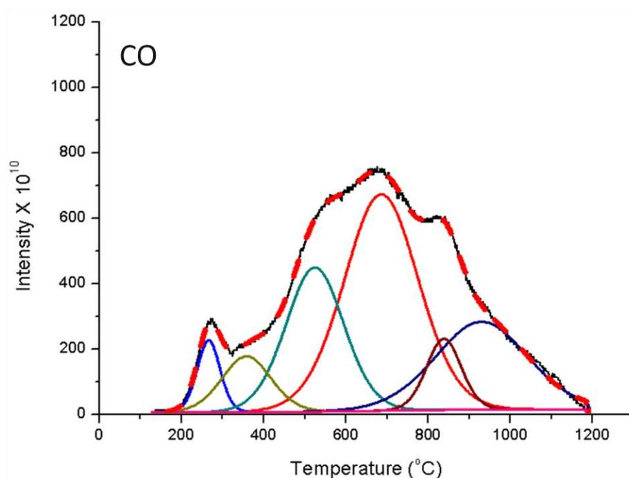
**Figure 4.16.** Results of deconvolution of TPD spectra (CO) from OAC4 without preset constraint for full width at half maximum
