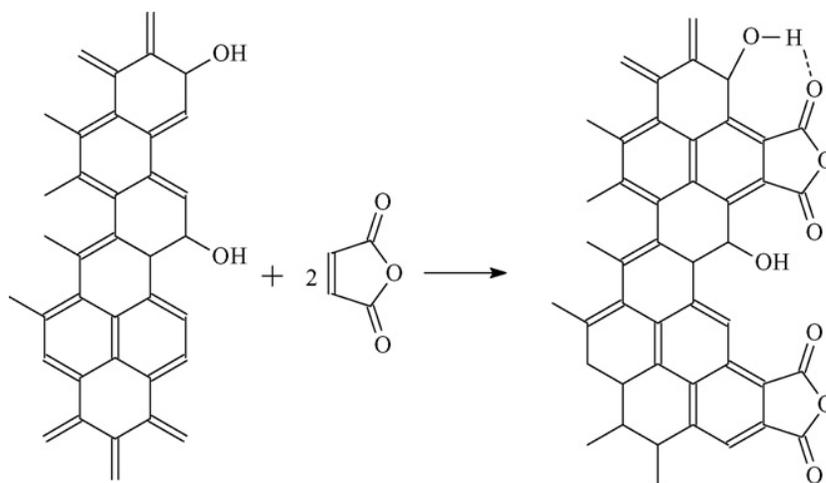
**Figure 1.3.** Schematic of the formation of new surface functional groups on carbon nanofiber by maleic anhydride (figure taken from Lu et al. [20]).
