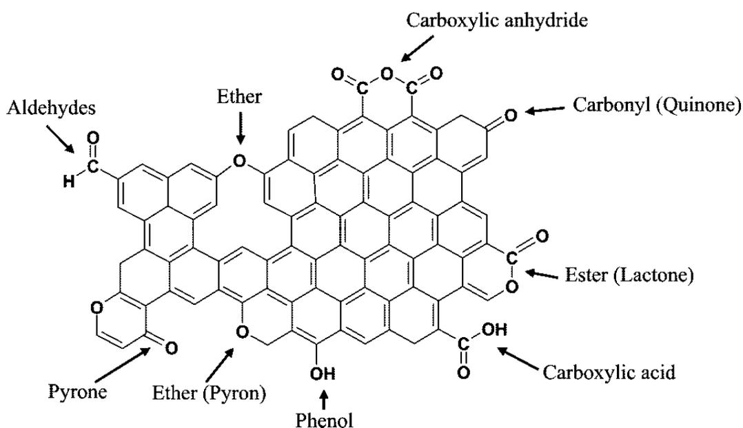
**Figure 1.1.** Oxygen functional groups on the surface of carbon materials (figure taken from Kundu et al. [24]).
