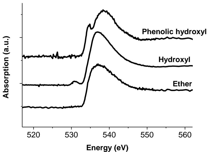
**Figure 4.7.** Oxygen K-edge XANES spectra of hydroxyl-type functional groups: (1) phenolic hydroxyl (PVP), (2) hydroxyl (PVA), and (3) ether (methyl cellulose)
