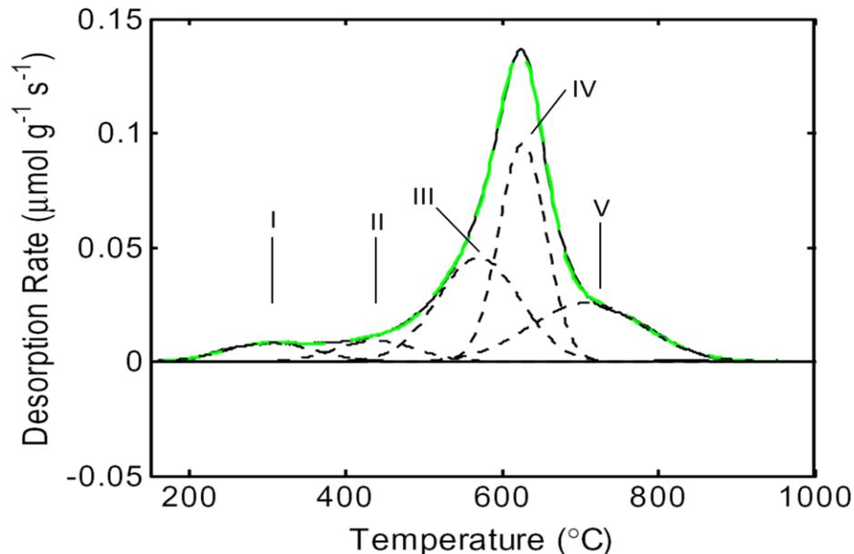
**Figure 2.3.** TPD spectrum of oxidized carbon nanofiber: (I) carboxyls, (II) carboxylic anhydrides, (III) peroxides, (IV) and (V) lactones at different sites (figure taken from Zhou et al. [47]).
