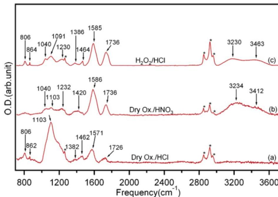
**Figure 2.2.** FTIR spectra of differently processed carbon nanotubes (figure taken from Kim et al. [45]).
