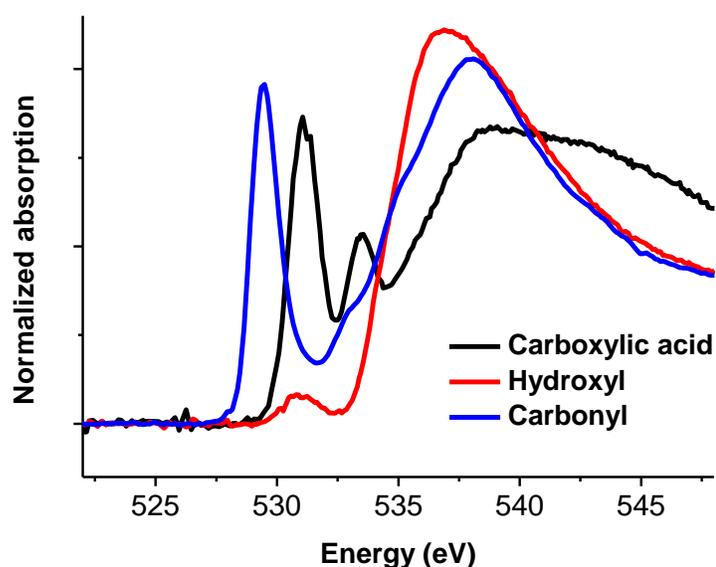
**Figure 4.9.** Normalized oxygen K-edge XANES spectra of carboxylic acid (PAA), hydroxyl (PVA), and carbonyl (anthrone)
