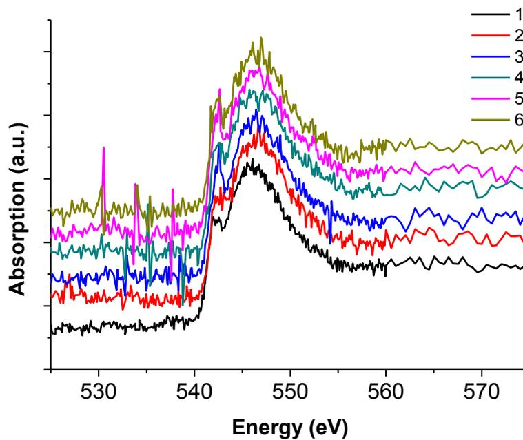
**Figure 4.4.** Multiple XANES spectra of PVP collected in fluorescence yield mode before merging
