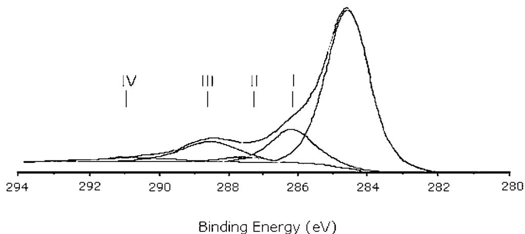
**Figure 2.1.** Deconvolution of XPS spectrum of oxidized carbon fiber: (I) phenols, (II) carbonyls, (III) carboxyls, (IV) carbonate (figure taken from Yue et al. [5]).
