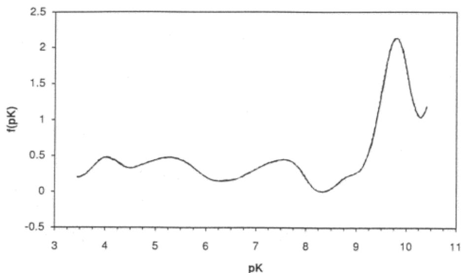
**Figure 2.4.** Acid constant distribution of an oxidized activated carbon (figure taken from Bandosz et al. [48]).
