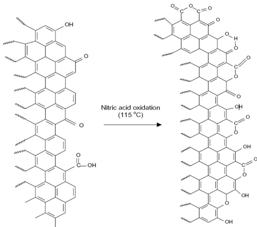
**Figure 1.2.** Schematic of the formation of new surface functional groups on carbon nanofiber by nitric acid oxidation (figure taken from Lakshminarayanan et al. [19]).
