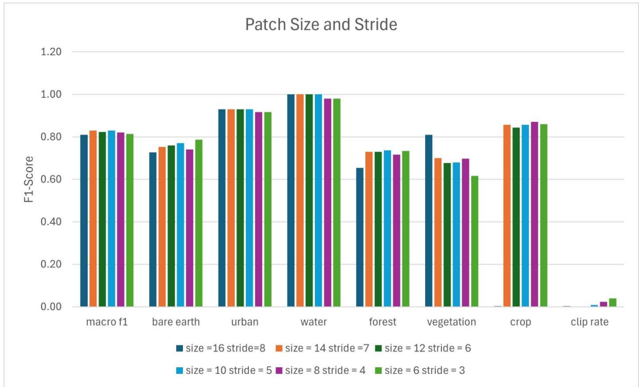
Figure 53 An ablation study showing how the F1-score changes for various values of patch size and patch stride.
