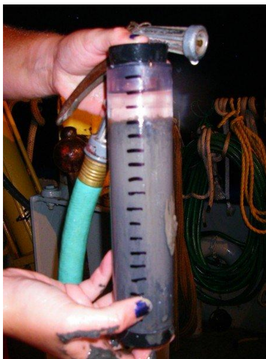
Fig. 4: Sub-cored surficial Lake Erie central basin sediment collected from the ship box core during 2007-08. These samples were used in the determination of algal pigment concentrations.
