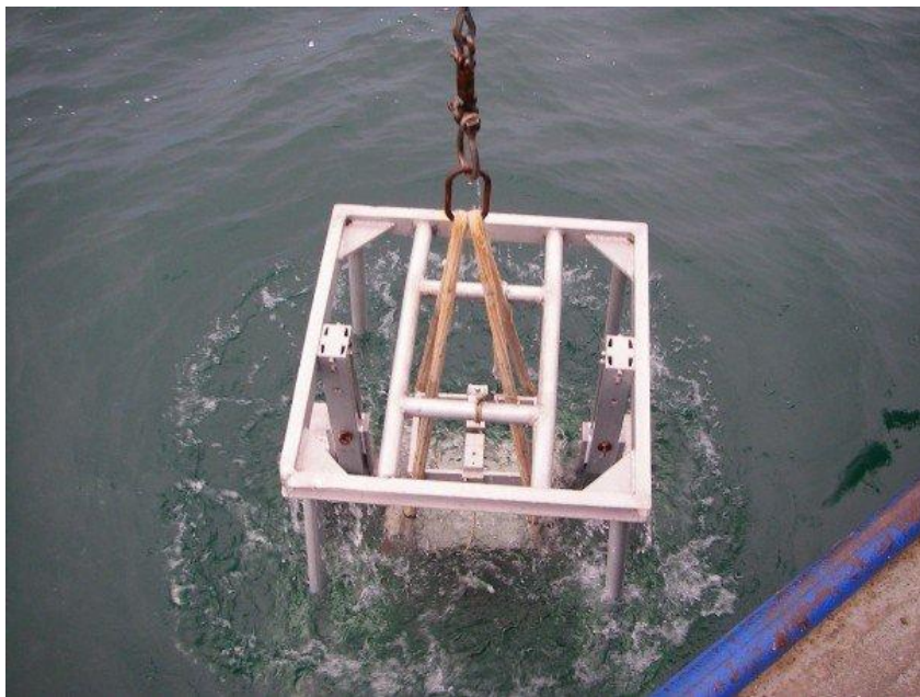
Fig. 3: Ship box core sampler (0.5 m 2 ) collecting surficial Lake Erie central basin sediments 2007-08.
