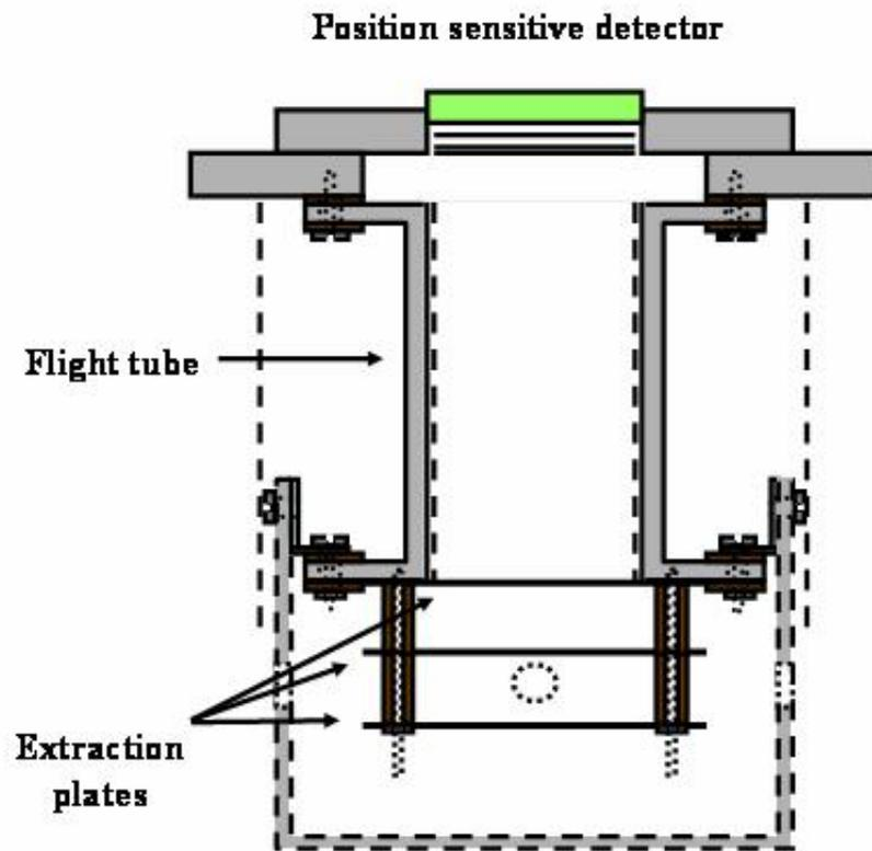
Figure 5.1: Cross-section of the velocity map imaging apparatus. The dashed lines represent magnetic shielding.
