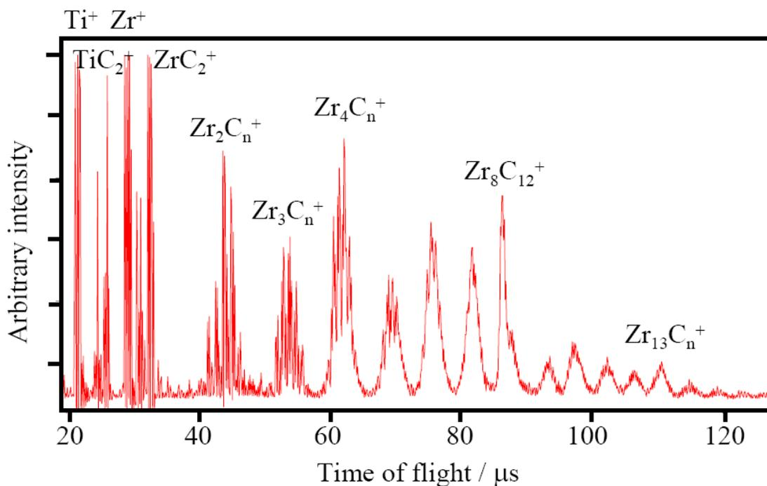
Figure 3.2: Mass spectrum of titanium:zirconium mixed metal-carbon clusters using a 50:50 Zr:Ti mixed metal alloy rod in a laser vaporization source coupled to a time-of-flight mass spectrometer. The rod is vaporized by the 2nd harmonic (532 nm) of a Nd:YAG laser. The clusters are ionized by a XeCl excimer laser (308 nm).
