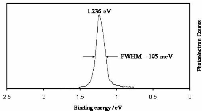
Figure 5.7: Photoelectron spectrum of photodetached electrons from copper anions. The full width at half max (FWHM) is 105 meV.
