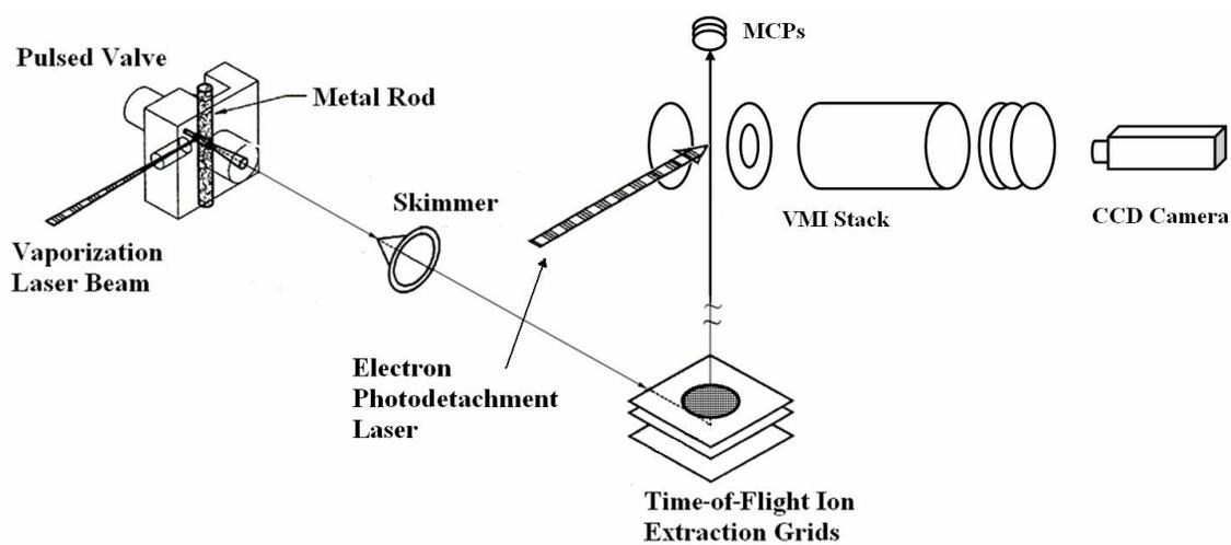
Figure 2.3: Diagram of the instrument following addition of velocity map imaging (VMI) stack. A laser vaporization source is coupled to an anion time-of-flight mass spectrometer, which is equipped with a velocity map imaging apparatus.
