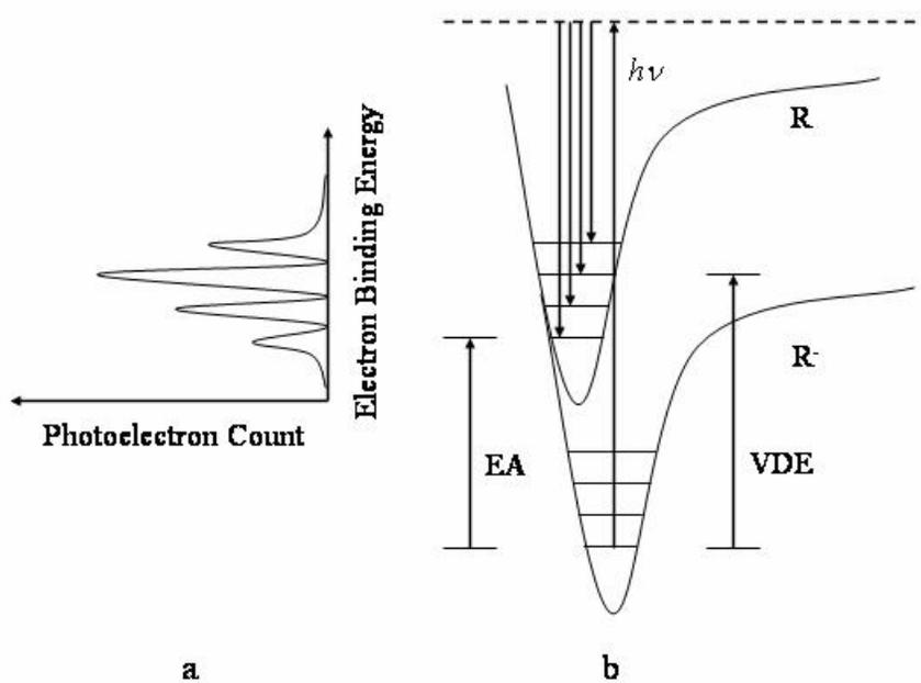
Figure 1.1: Qualitative diagram displaying the resulting photoelectron spectrum (a) of a photodetached electron following excitation from the ground state of  $R^-$  to a virtual level in the  $R + e^-$  continuum by a photon of fixed energy,  $h\nu$  (b). The electron affinity (EA) of R and the vertical detachment energy (VDE) of  $R^-$  are labeled. Adopted from Ervin and Lineberger.[17]
