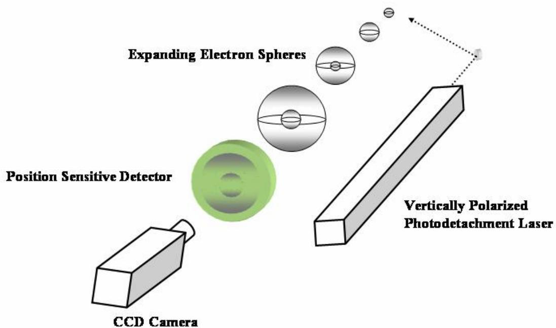
Figure 1.2: Diagram portraying the expanding electron spheres that contain information regarding the kinetic energy of the photodetached electron as they travel toward a position sensitive detector in the velocity map imaging apparatus. The larger sphere represents electrons with a given kinetic energy higher than the electrons contained within the smaller sphere.
