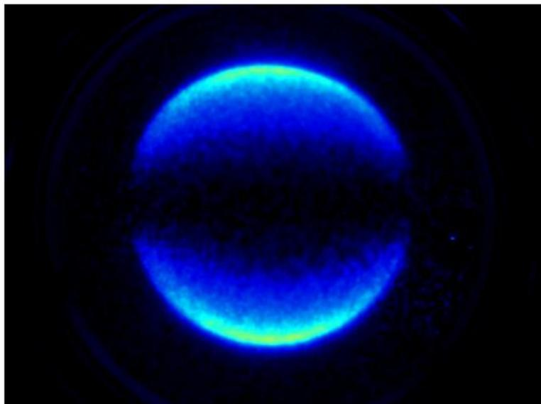
Figure 5.5: Raw image of photodetached electrons from copper anions.
