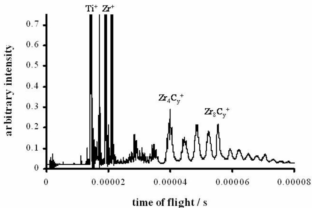
Figure 4.1: Time-of-flight mass spectrum of cations detected following excitation of a neutral molecular beam of  $\text{Ti}_x\text{Zr}_y\text{C}_z$  clusters with a XeCl excimer laser (308 nm).
