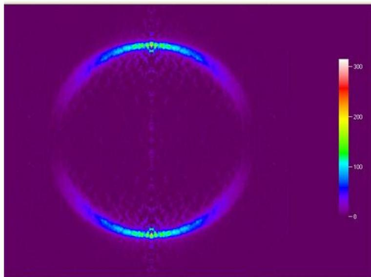
Figure 5.6: Reconstructed image of photodetached electrons from copper anions using the BASEX Abel transform method.
