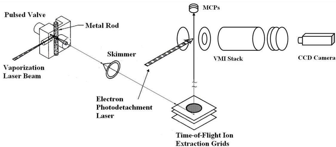
Figure 5.4: Diagram of the instrument following addition of velocity map imaging (VMI) stack. A laser vaporization source is coupled to an anion time-of-flight mass spectrometer, which is equipped with a velocity map imaging apparatus.
