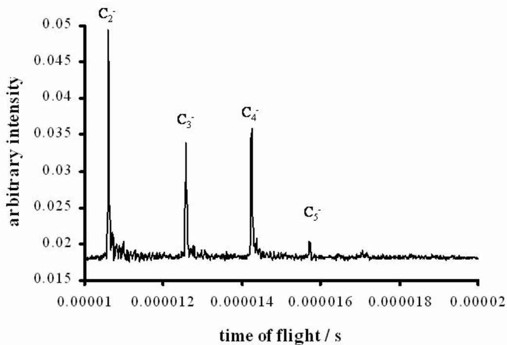
Figure 4.2: Time-of-flight mass spectrum of anions detected following excitation of a neutral molecular beam of  $Ti_xZr_yC_z$  clusters with a XeCl excimer laser (308 nm).
