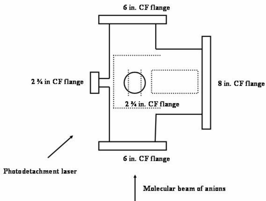
Figure 5.3: Custom chamber that contains the velocity map imaging stack. The photodetachment laser enters the chamber perpendicular to the page through the two  $2\frac{3}{4}$  in. Conflat (CF) flanges (the exit  $2\frac{3}{4}$  in. is not shown in this diagram).
