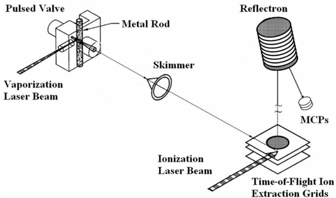
Figure 2.1: Diagram of the instrument prior to modifications. A laser vaporization source is coupled to a reflectron time-of-flight mass spectrometer.
