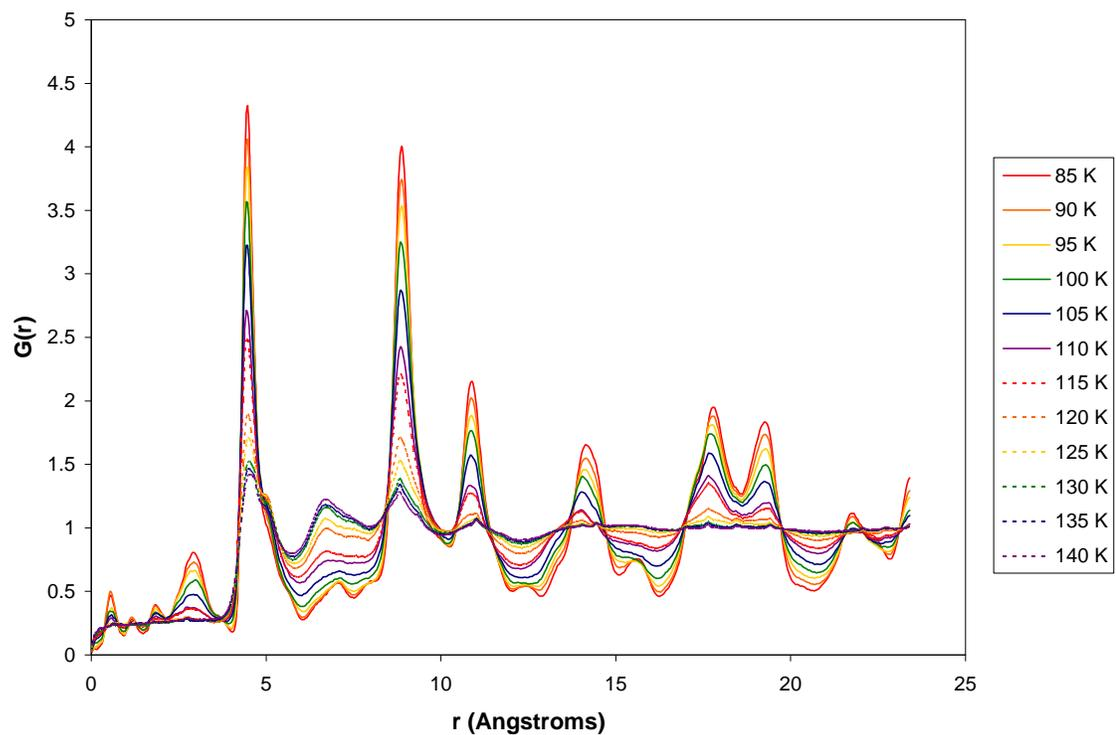
Figure 4-4: Radial Distribution Function of Pentane on Graphite
