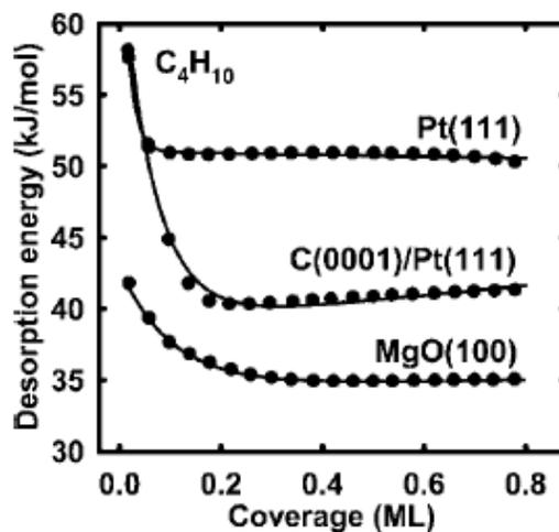
Figure 6-15: Desorption Energy as a Function of Coverage [10]
