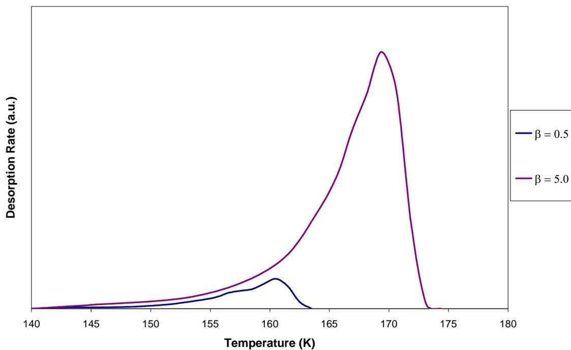
Figure 6-11: TPD Profiles –  $\beta = 0.5$  K/s and  $\beta = 5.0$  K/s, Monolayer Initial Coverage
