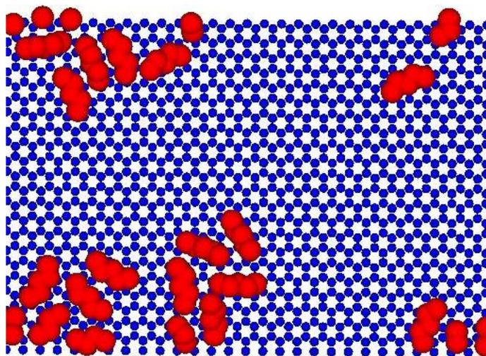
Figure 5-5: Molecular Configuration of Pentane on the Basal Plane of Graphite at 0.25 ML and 165 K
