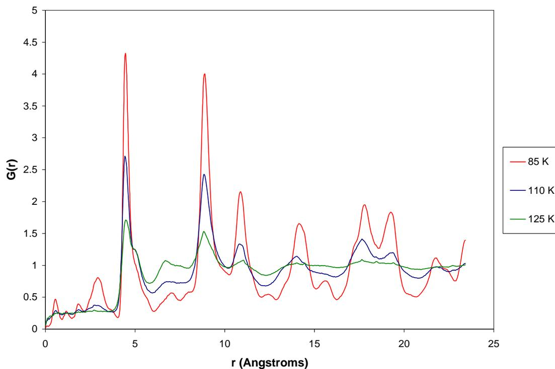
Figure 4-5: Radial Distribution Function of Pentane on Graphite – Select Temperatures
