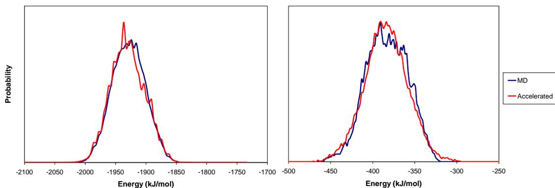
Figure 5-1: Energy Histograms for Pentane Desorbing from the Basal Plane of Graphite: From Left to Right: Molecule-Surface Energy for Monolayer Coverage at 160 K, Intermolecular Energy for 0.5 Monolayer Coverage at 160 K
