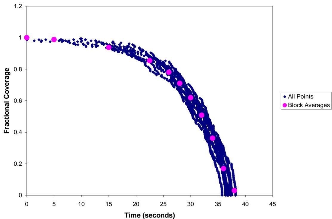
Figure 6-4: Fractional Coverage versus Time – Monolayer Coverage,  $\beta = 0.6$  K/s, Multiple Simulations and Block Averages
