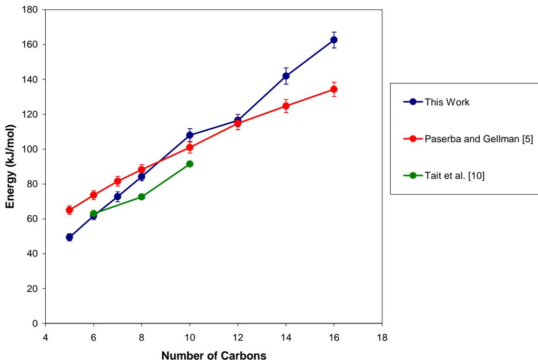
Figure 3-8: Desorption Energy Comparison – Simulated and Experimental
