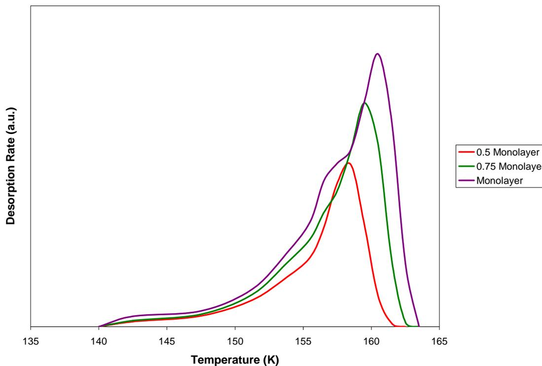
Figure 6-8: TPD Profiles – Variable Initial Coverage,  $\beta = 0.5$
