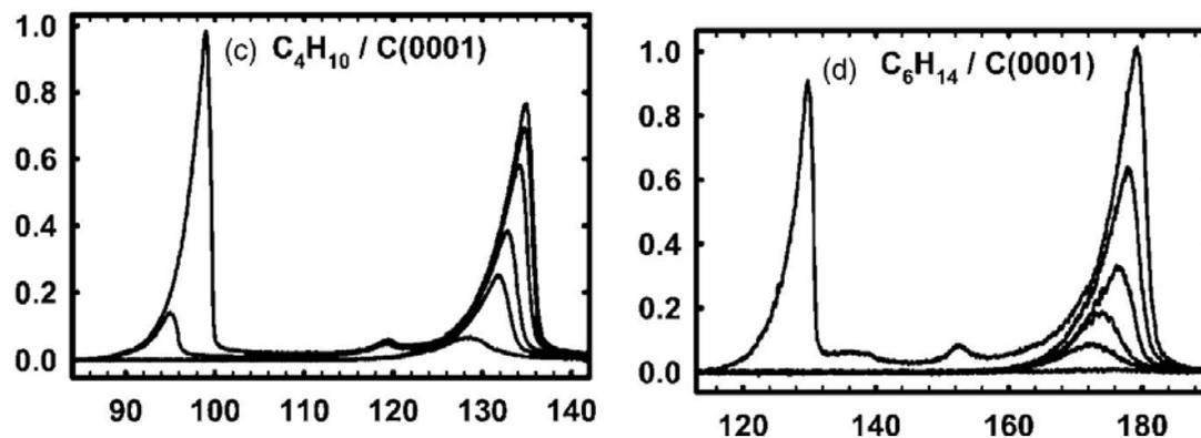
Figure 6-7: TPD Profile for Butane and Hexane Desorbing from the Basal Plane of Graphite [10]
