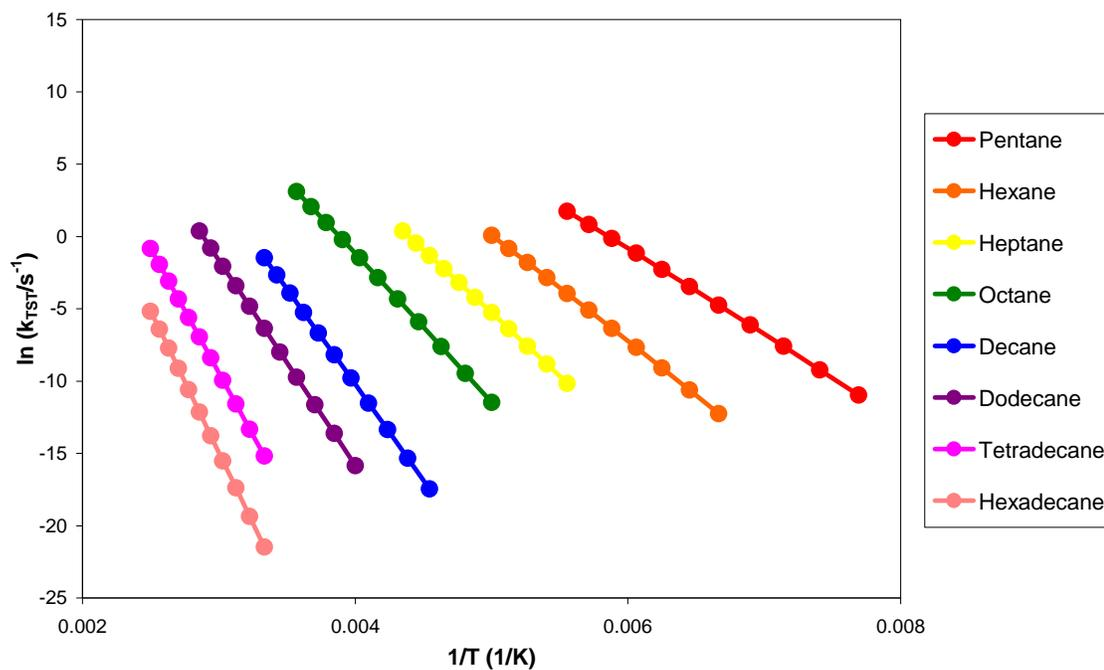
Figure 3-4: Arrhenius Plots – Variable Chain Length
