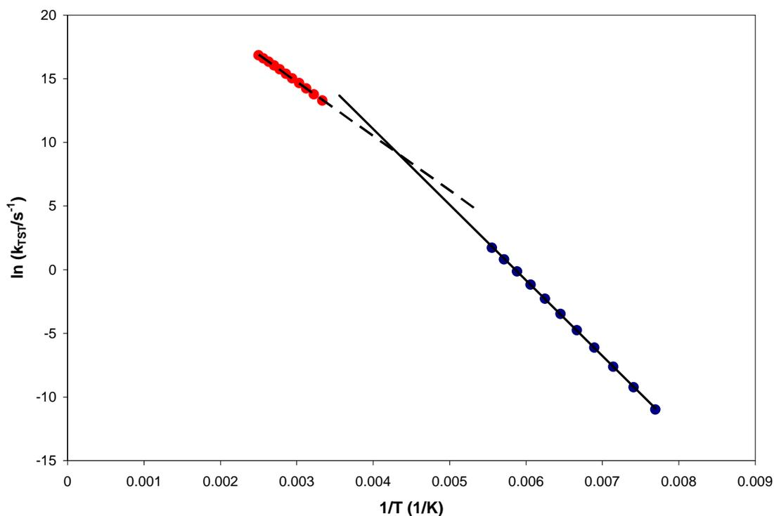
Figure 3-14: Arrhenius Plot for Pentane – Variable Temperature Range
