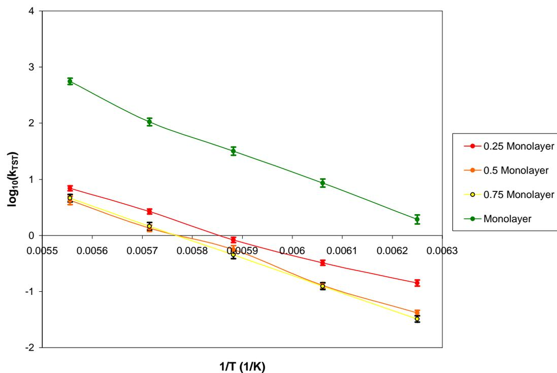
Figure 5-4: Arrhenius Plots of the Desorption of Pentane from the Basal Plane of Graphite – Variable Coverage
