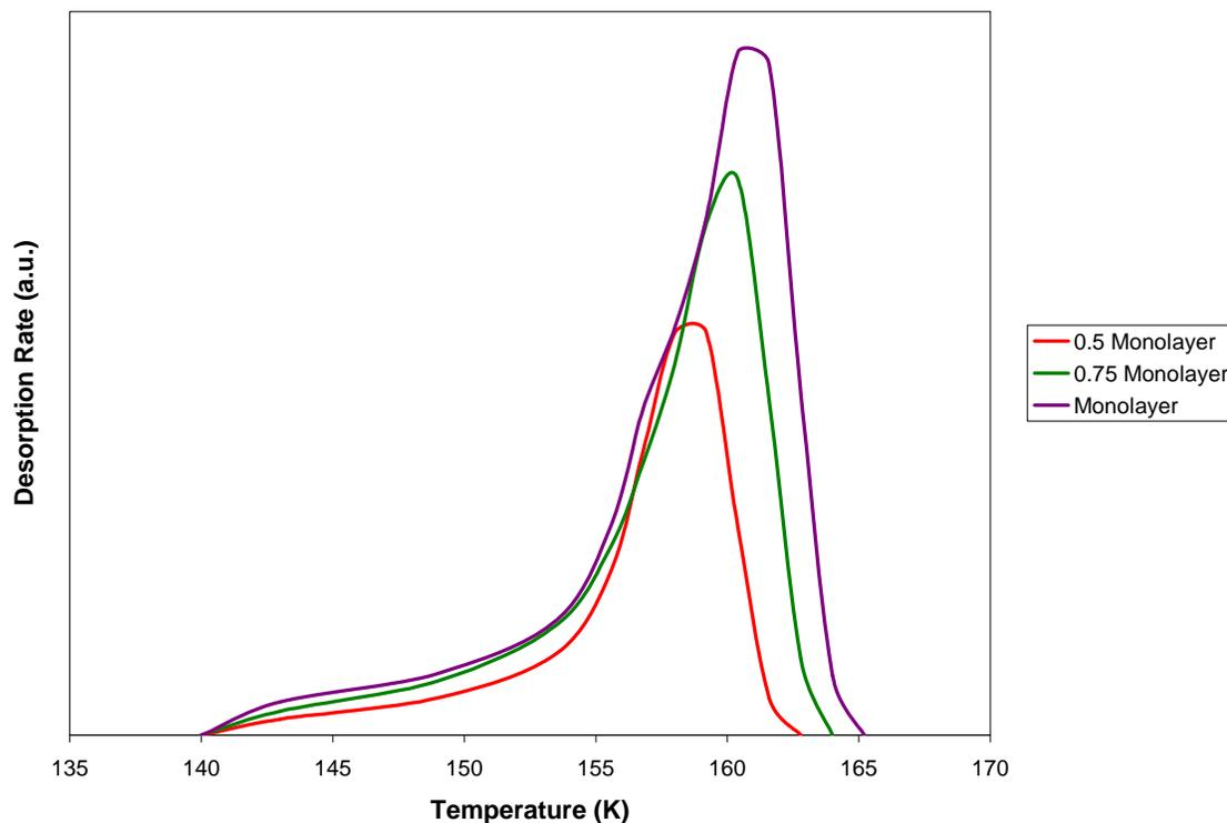
Figure 6-6: TPD Profiles – Variable Initial Coverage,  $\beta = 0.6$
