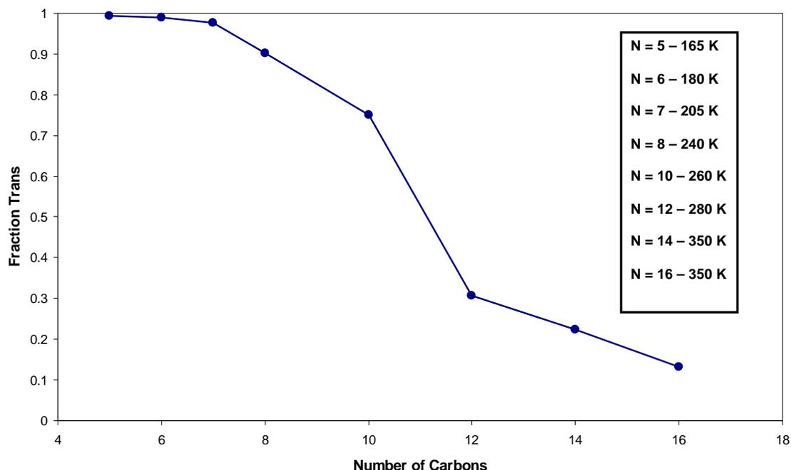
Figure 3-10: Fraction Trans as a Function of Chain Length
