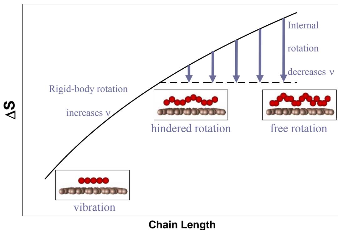
Figure 3-12: Schematic of the Effect of Chain Length on Entropy and Prefactor
