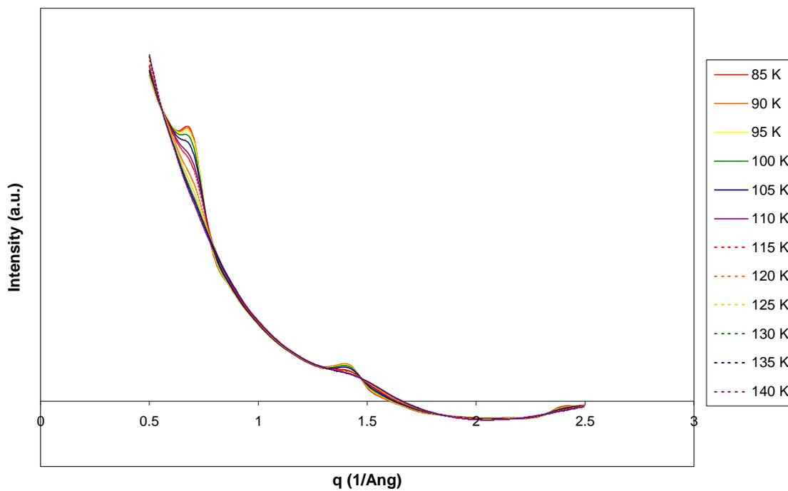
Figure 4-2: Neutron Scattering Intensity of Pentane on Graphite
