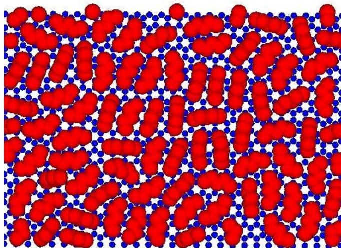
Figure 5-6: Molecular Configuration of Pentane on the Basal Plane of Graphite at Monolayer and 165 K
