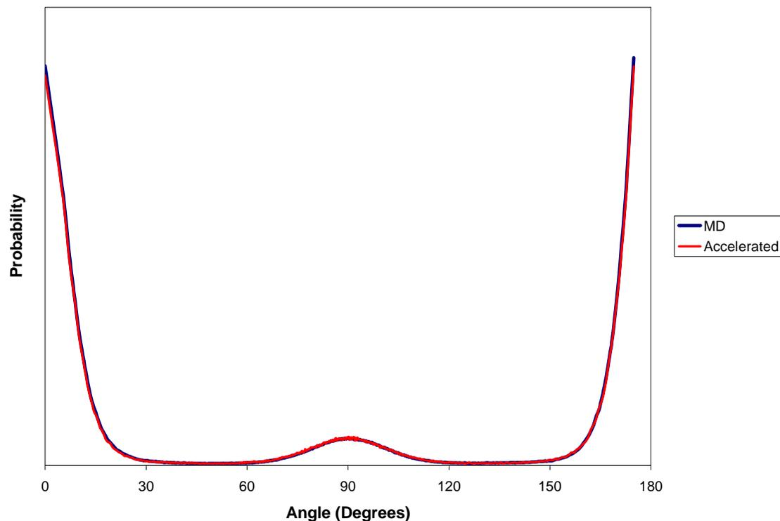
Figure 5-3: Roll Angle Distribution for Pentane on the Basal Plane of Graphite – Monolayer Coverage at 170 K
