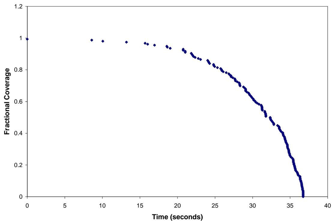
Figure 6-2: Characteristic Plot of Fractional Coverage versus Time – Monolayer Coverage,  $\beta = 0.6$  K/s, Single Simulation
