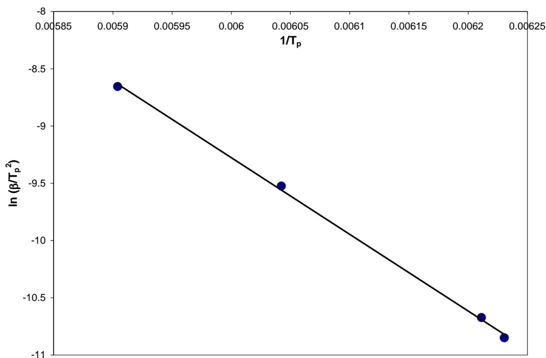
Figure 6-13: Variable Heating Rate Plot of  $\ln(\beta/T_p^2)$  versus  $1/T_p$
