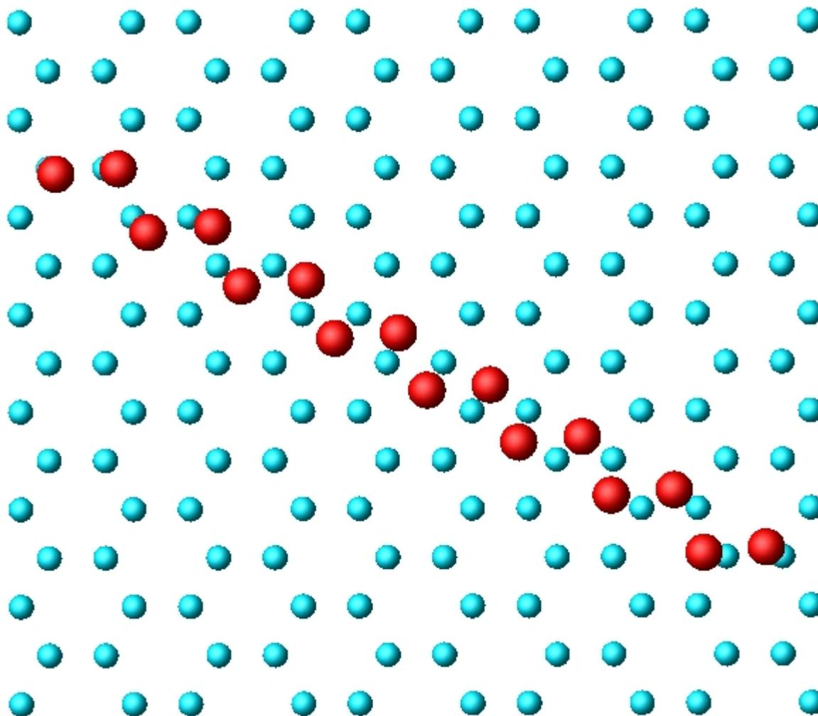
Figure 3-7: Minimum Energy Configuration for Hexadecane (Hydrogen Atoms Omitted for Clarity)
