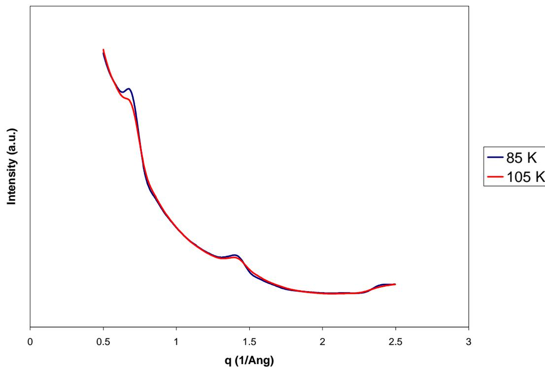
Figure 4-3: Neutron Scattering Intensity of Pentane on Graphite – Select Temperatures
