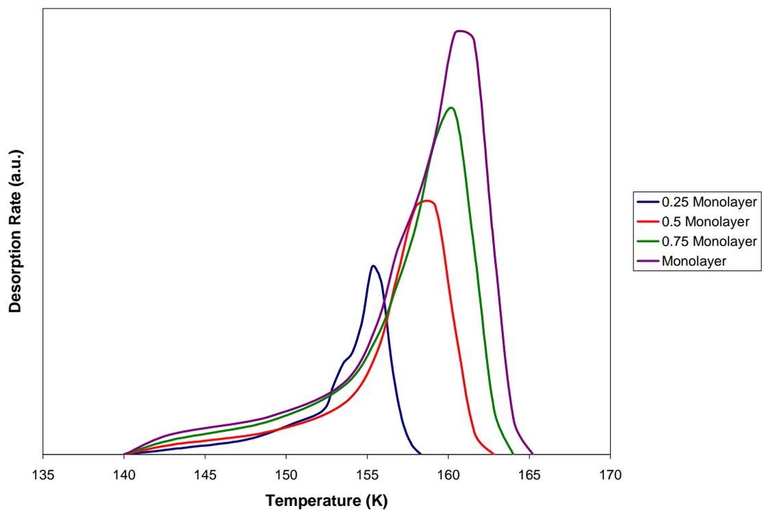
Figure 6-14: TPD Profiles – Variable Coverage (Including 0.25 ML),  $\beta = 0.6$  K/s
