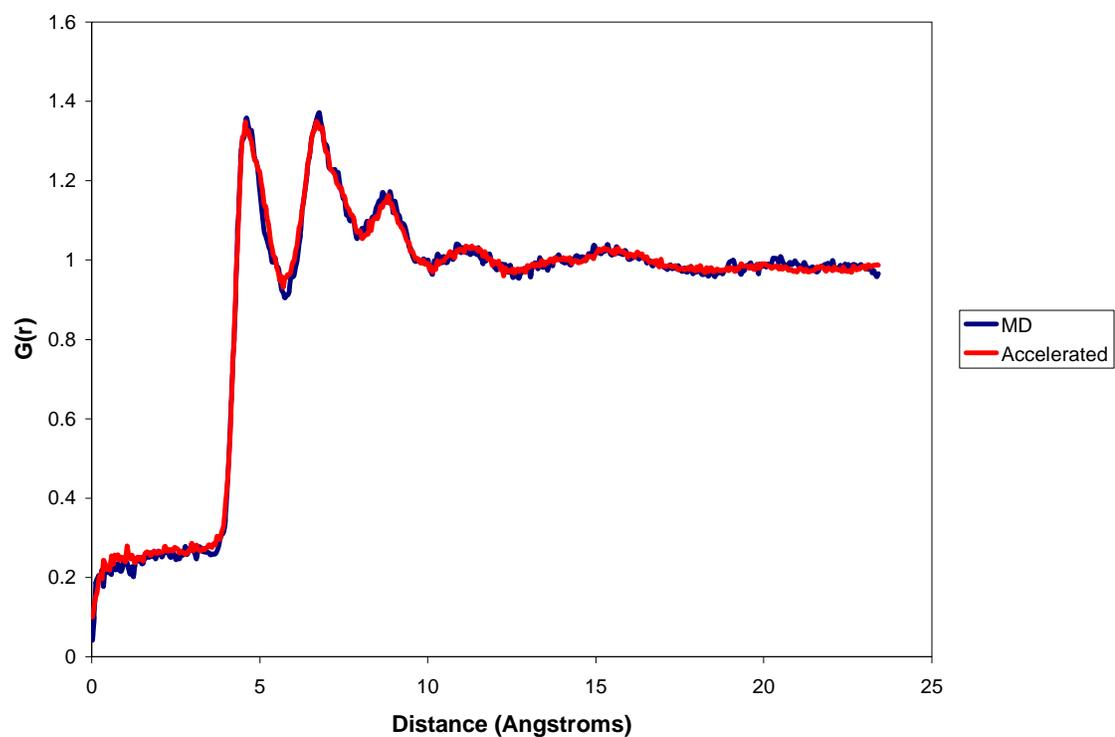
Figure 5-2: Radial Distribution Function of Pentane on Graphite – 0.75 Monolayer, 170 K
