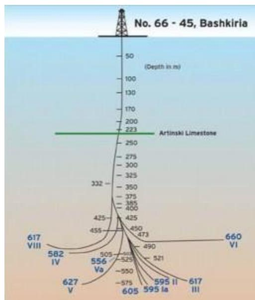
**Figure (2.1): The first multilateral well (66/45), From Reference (Bosworth et al, 1998)**
