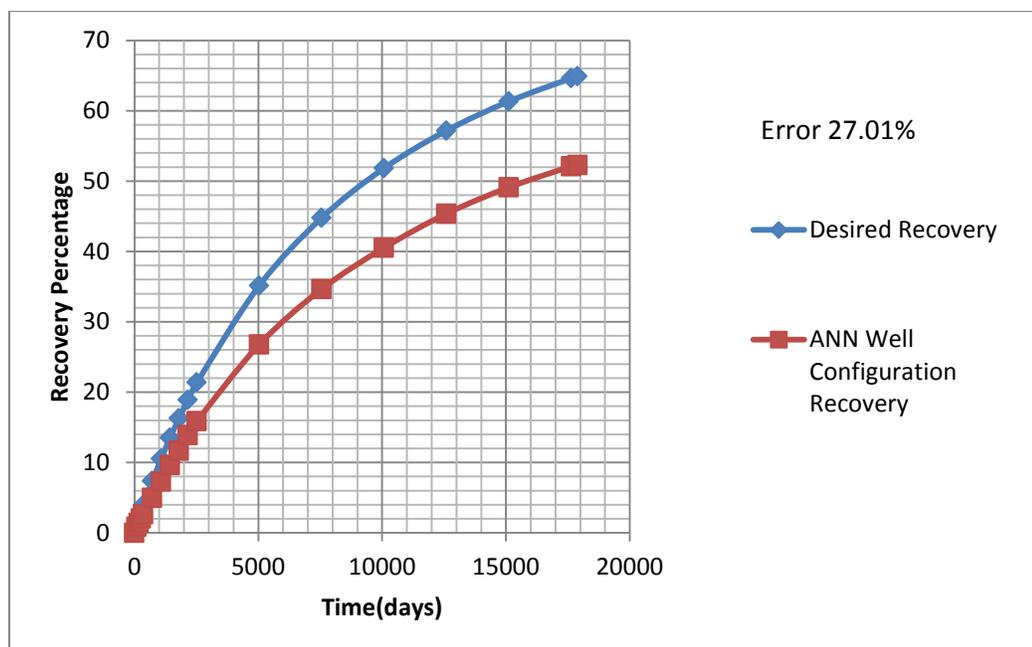
Figure (6.16): Sample result from 500-case study with  $\text{error} > 15\%$  (Inverse network)
