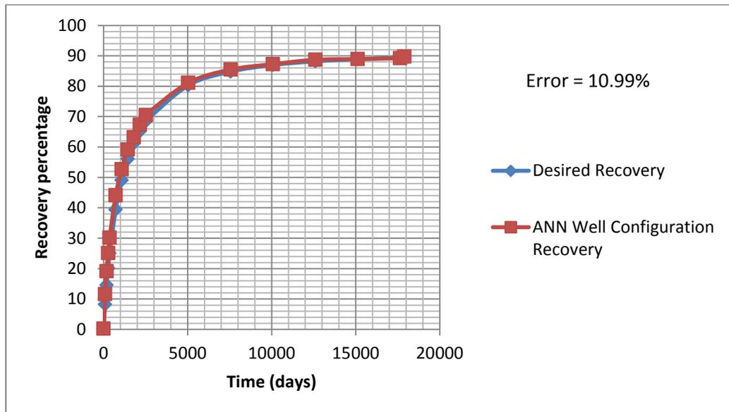
Figure (6.5): Sample result from 50-case study with  $10\% < \text{error} < 15\%$  (Inverse network)
