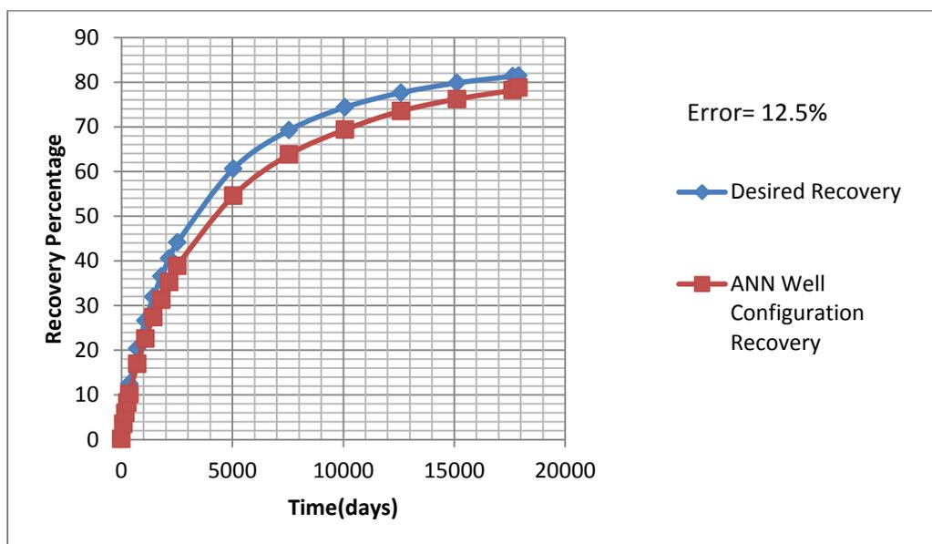
Figure (6.15): Sample result from 500-case study with  $10\% < \text{error} < 15\%$  (Inverse network)
