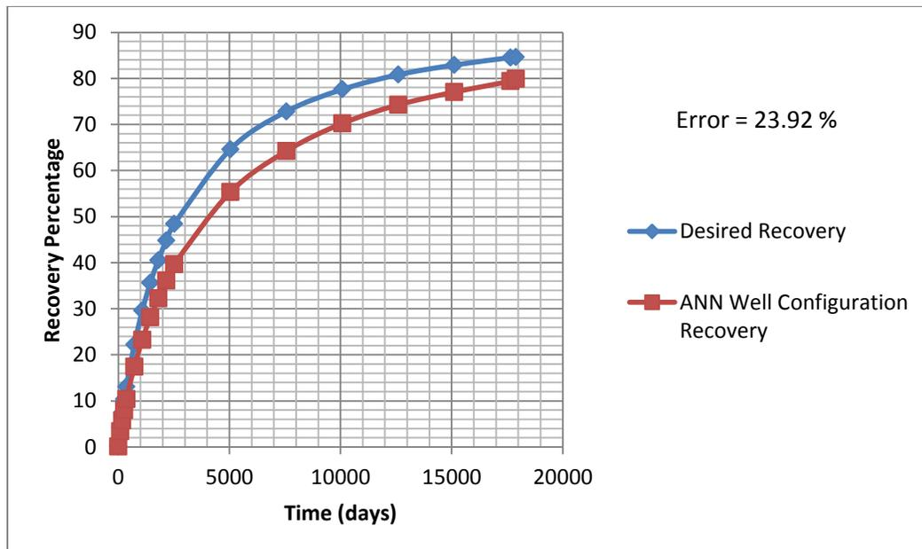
Figure (6.6): Sample result from 50-case study with  $\text{error} > 15\%$  (Inverse network)
