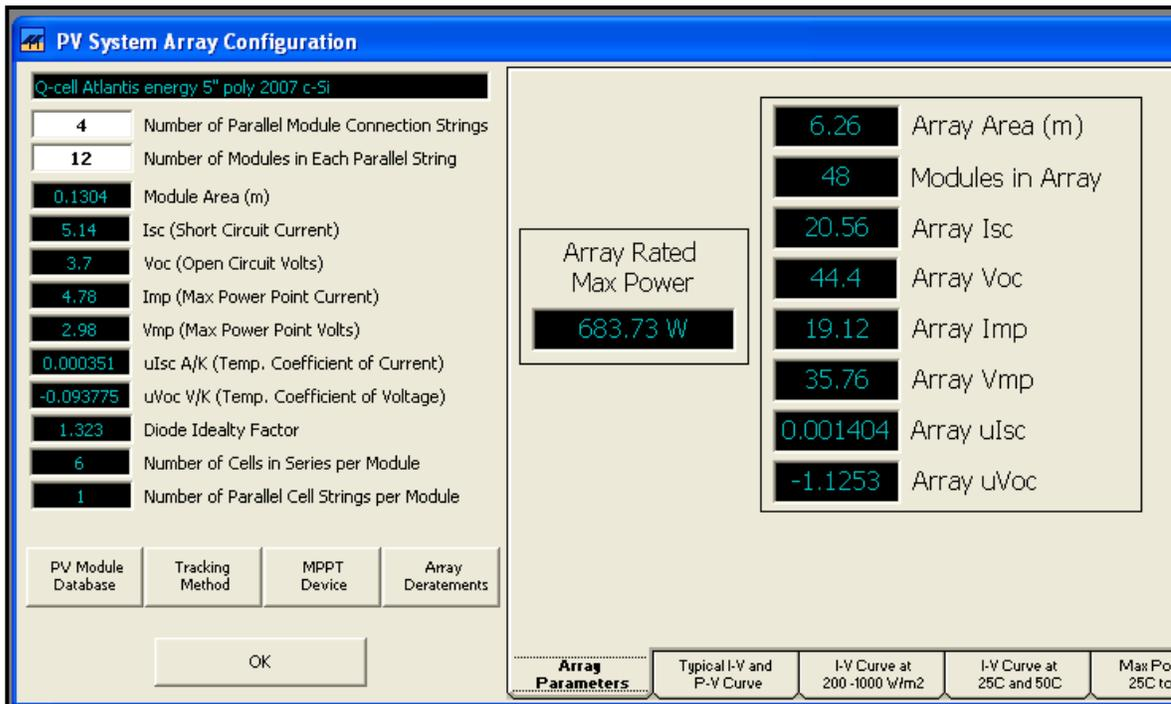
Figure 6-3: PV array configuration
