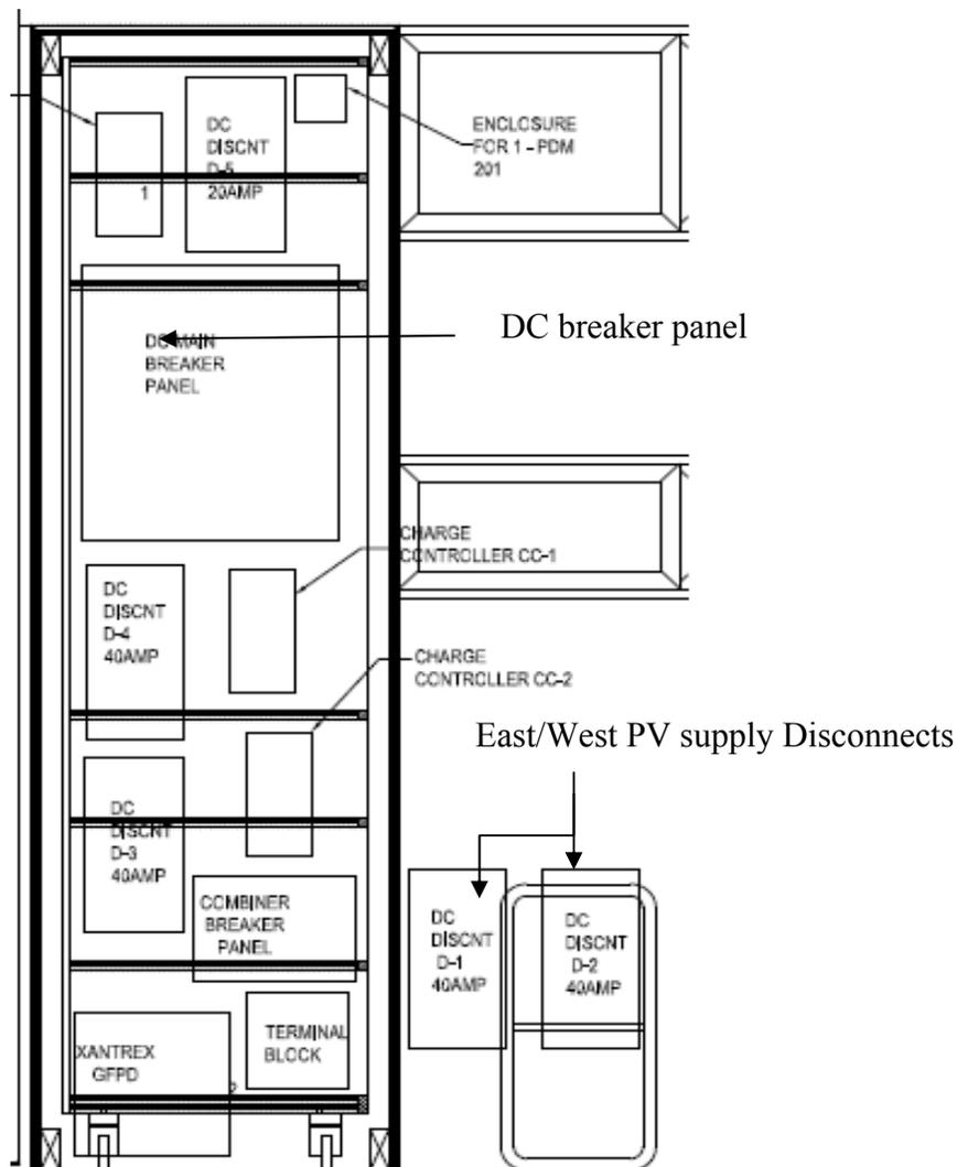
Figure 5-1: DC Equipment elevation on the east interior wall
