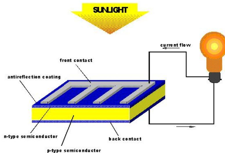
Figure 2-2 Operation of a PV cell (Source School of Photovoltaic and Renewable engineering, New South Wales, 2008)
