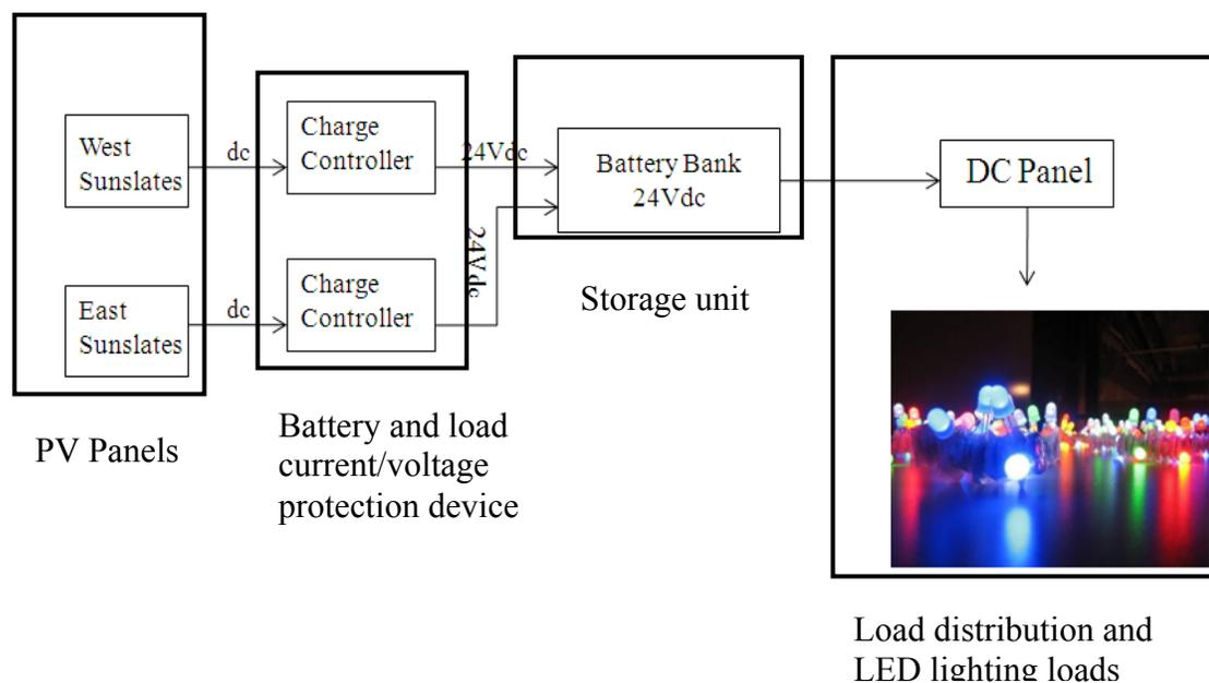
Figure 4-6: A block diagram of the DC LED lighting system
