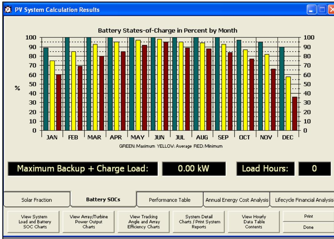
Figure 6-7: Battery state of charge (SOC) in percentage per month
