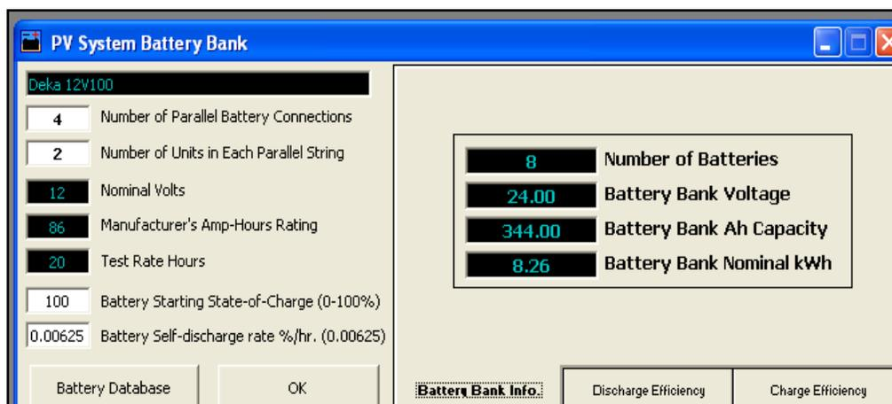
Figure 6-6: PV system battery bank details
