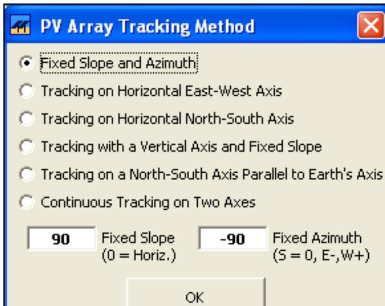
Figure 6-4: East PV Array tracking method
