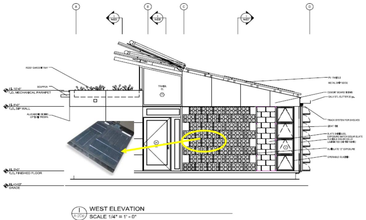
Figure 4-4: Solar slates mounted vertically on the west wall of the Solar house
