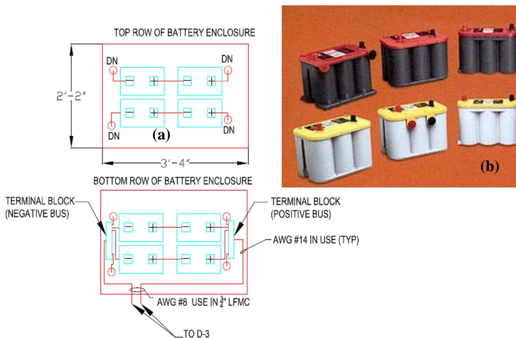
Figure 5-4: (a) 24VDC Battery wiring detail (b) Photograph of batteries
