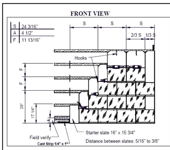
Figure 5-3 (b) A front view section on batten installation and slate
