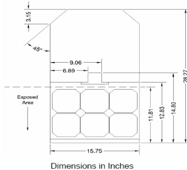
Figure 4-5: Physical dimensions of each solar slate
