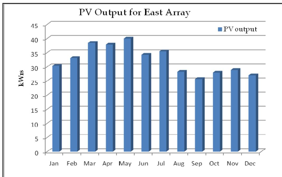
Figure 6-9: East array PV output
