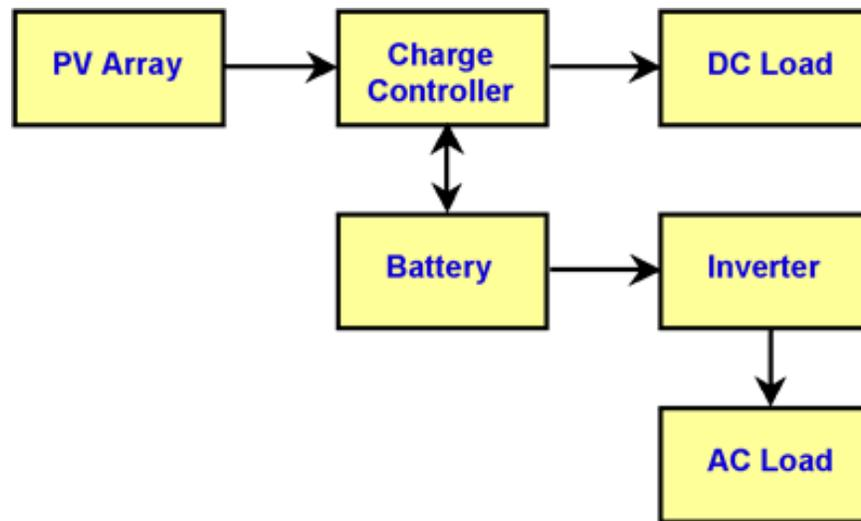
Figure 2-3 Typical PV stand-alone AC system (Source Florida Solar energy center, 2007)
