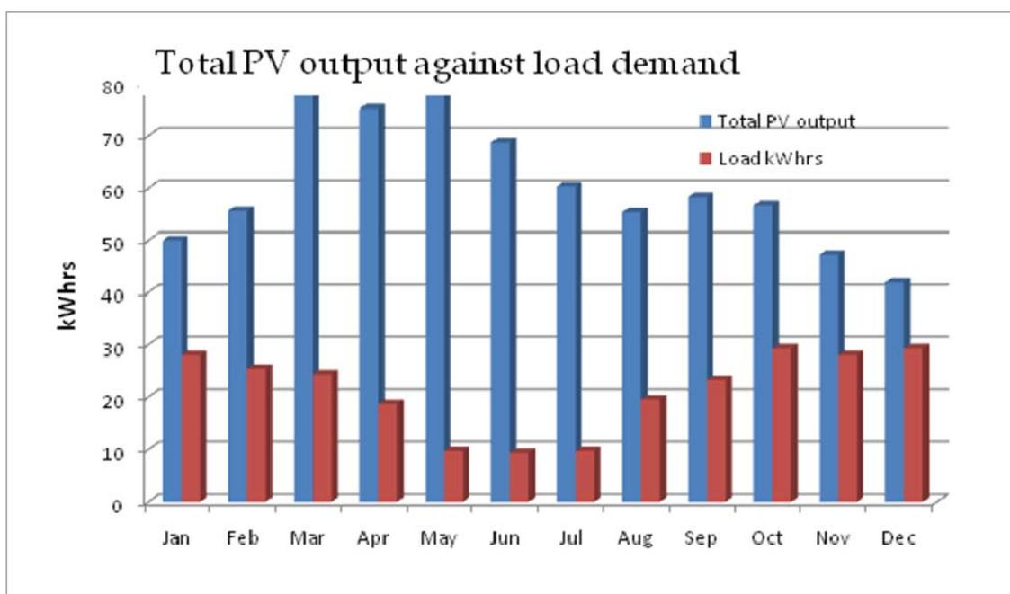
Figure 6-11: Total PV Output against load demand (in kWhrs)
