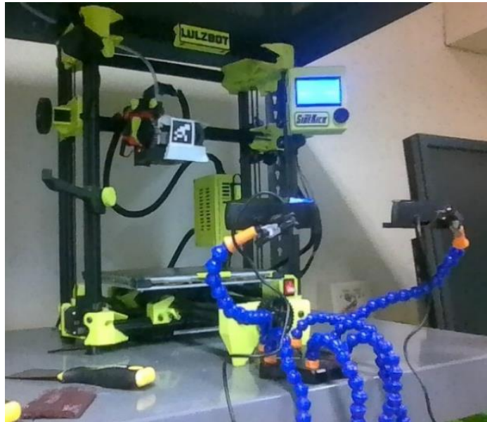
Figure 15. Rapid ArUco marker based dual-camera tracking deployment. (Top) true positions vs. calculated positions of the nozzle in the xz plane. (Bottom) the camera and marker setup on a Lulzbot Taz Sidekick.
