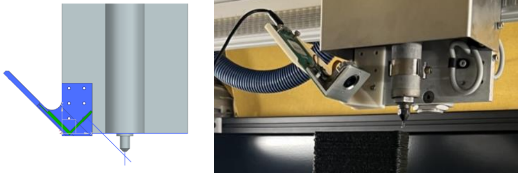
Figure 3. Thermal camera mounted on nozzle, showing design (left) and actual mount (right).
