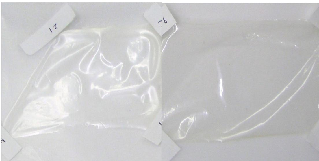
Figure 55 - Photographs of the SiO<sub>2</sub>-P(VDF-CTFE) hybrids. Left - 0.00 wt. %. Right - 3.38 wt. %.
