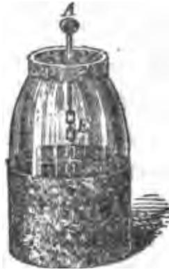
Figure 1 - Leyden jar. Note the foil covering and chain electrode inside the jar. Source: Reference 4.
