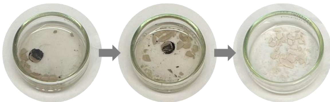
Figure S4-11: Optical images of the separation process where spent LLZO-SE and LFP were soaked in dimethylformamide followed by rinsed with dimethoxyethane to remove the polymer-salt layer along with a significant portion of lithium dendrites located near the surface of spent LLZO-SE.
