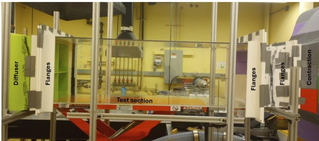
Figure 4-20: Flanges assembled onto the Wind Tunnel with adhesive tape.
