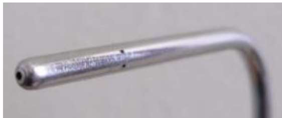
Figure 2-2: A detailed view of a Pitot-static probe reveals the presence of a stagnation pressure hole along with two static circumferential pressure holes [16].
