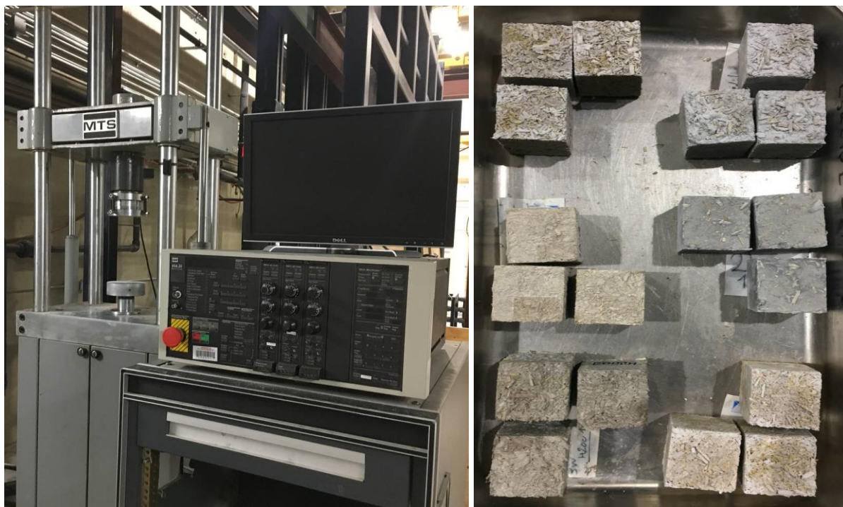
Figure 3-14. MTS Compressive Strength Test Assembly and Hempcrete Cubes to be tested.
