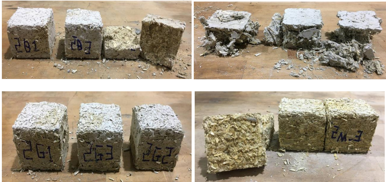
Figure 4-4. Post-Compression Test Form of 2B, 2F, 2G and 2M Hempcrete Specimens; Deformed & Crushed
