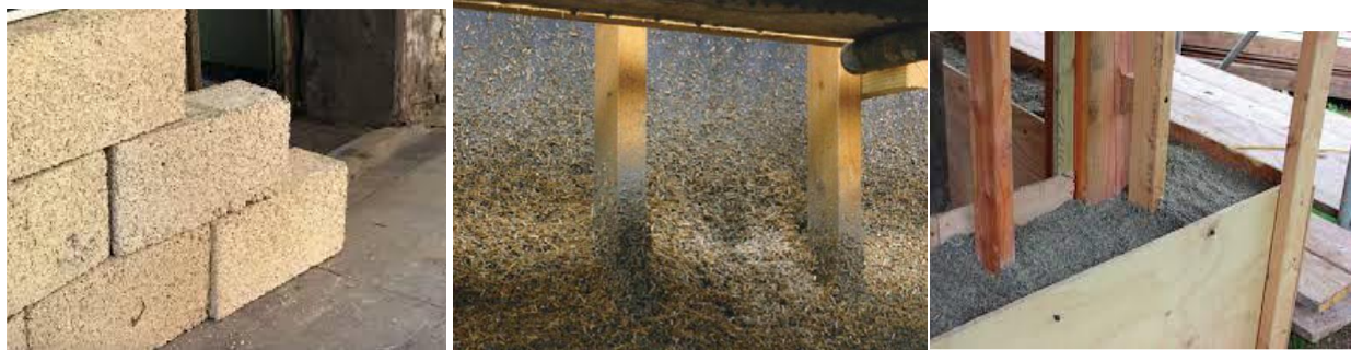
Figure 2-2. Different forms of Hempcrete. Adapted from [28].
