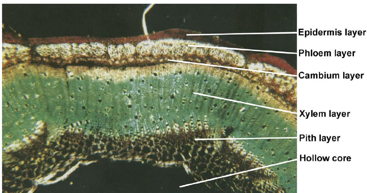
Figure 2-4. An optical micrograph of a hemp stem. Adapted from [39].
