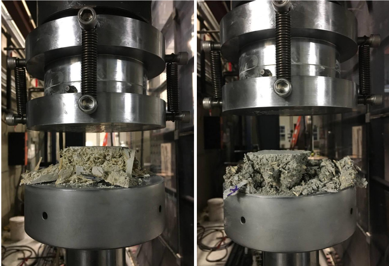
Figure 3-15. Hempcrete Cube under Compression Test Load
