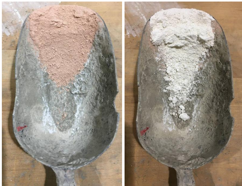
Figure 3-4. Highly Reactive Metakaolin Pozzolan material obtained from two different supplier; BURGESS OPTIPOZZ & R-E-D Industrial Products.
