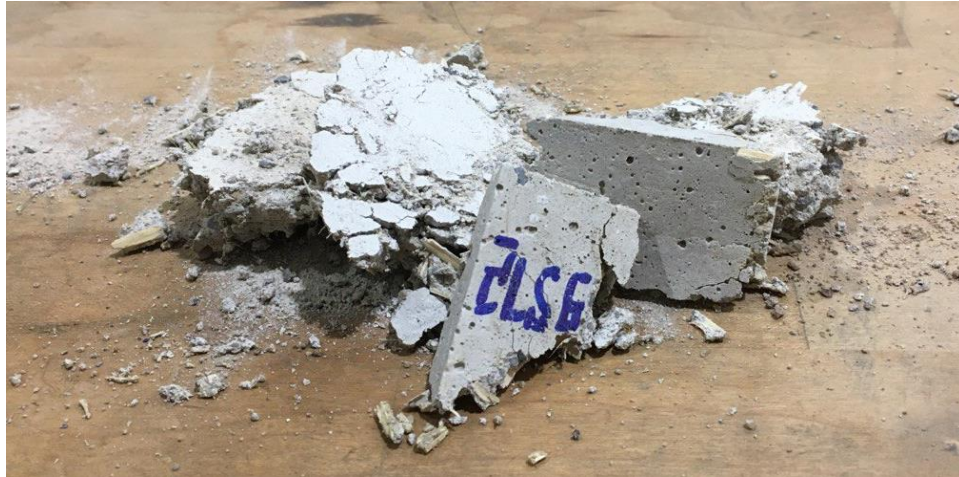
Figure 4-11. Crushed Forms of 2KMF50 & 2LS60 Hempcrete Specimens Under Compression Test
