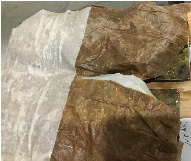
Figure 3-12. Casted Hempcrete Paste in Molds being Wrap in Damp Cloths
