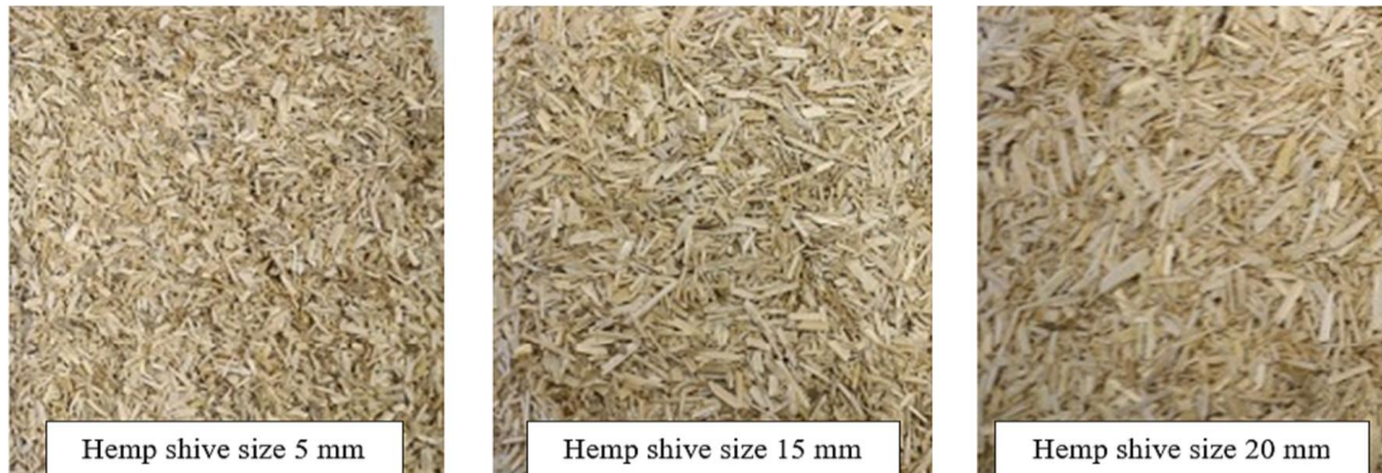
Figure 2-5. Hemp shives with different sizes. Adapted from [40].
