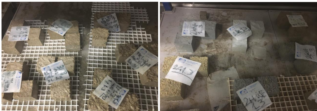
Figure 3-13. Demolded Specimens in Curing Chamber
