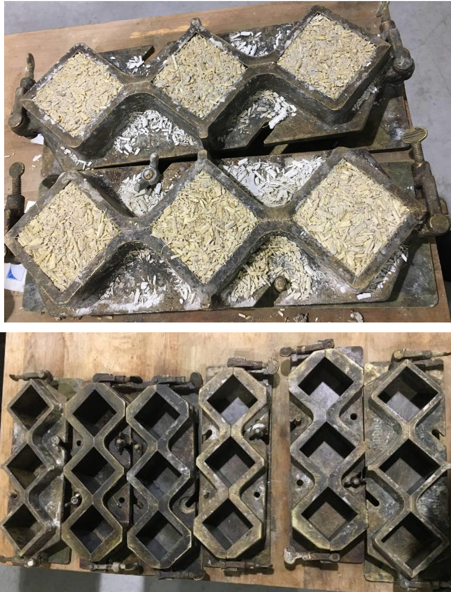
Figure 3-11. Molds being used for casting hempcrete mixtures
