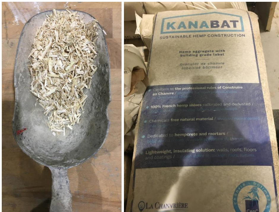
Figure 3-3. Hemp Hurd obtained from; La Chanvrière de l'Aube, branded as KANABAT.
