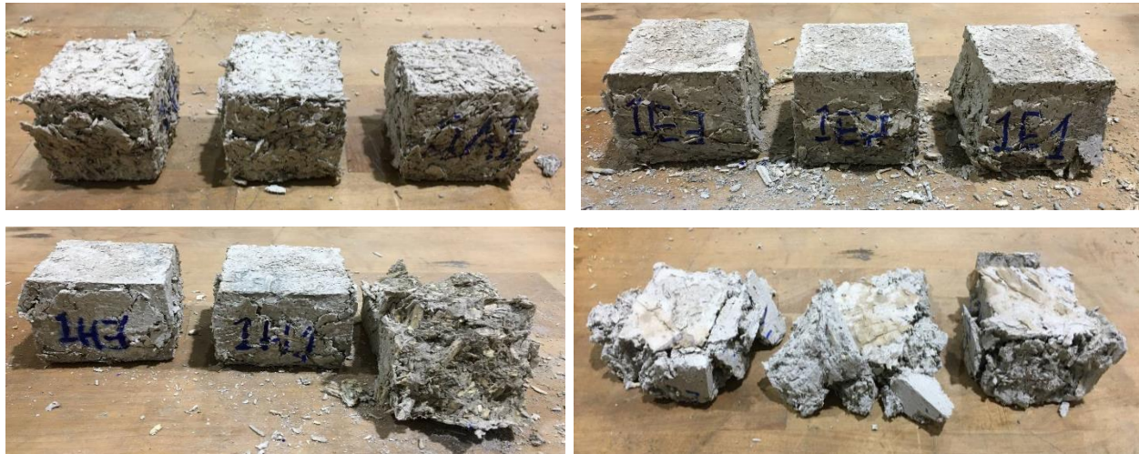
Figure 4-2. Post-Compression Test Form of 1A, 1E, 1H and 1L Hempcrete Specimens; Deformed & Crushed
