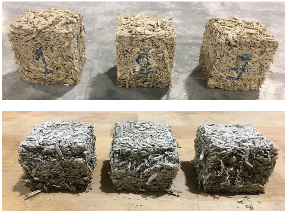
Figure 4-3. Undeformed and Deformed Shape of H1 Specimen made from Hemp Hurds, Hydrated Lime and Water with Ratios of 1:1:1
