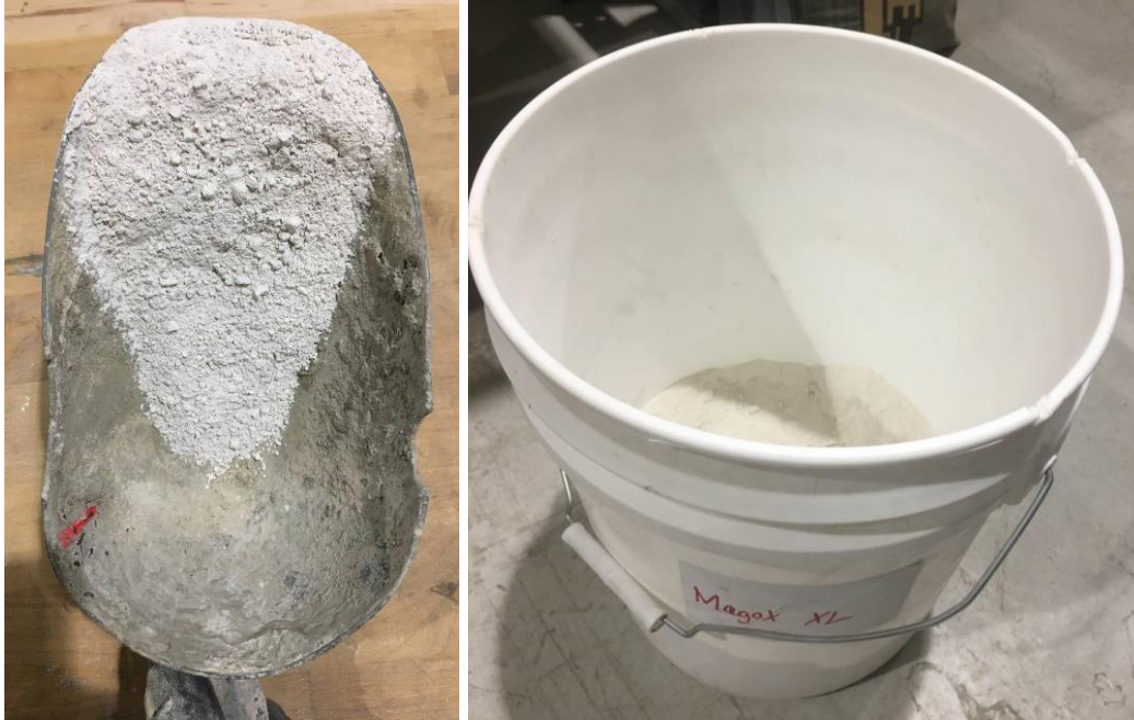
Figure 3-2. Premier Magnesia MgO-Cement; Magox XL used in Hempcrete Mixture
