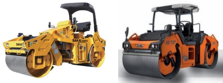
Figure 4-3 Static roller compactor (left) and oscillatory roller (right) in the Altoona project
