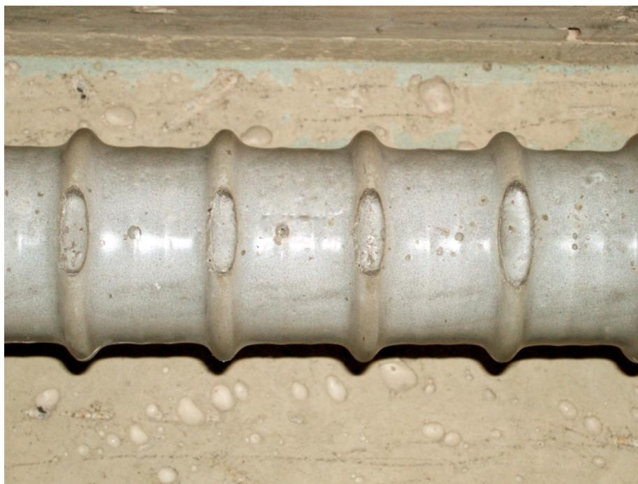
Figure 6-2: Close-Up of Air Pockets Along Peaks of Duct Ribs
