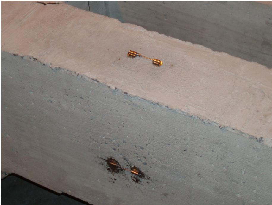
Figure 4-10: Vibrating Wire Strain Gauge Orientation on Beam Specimens
