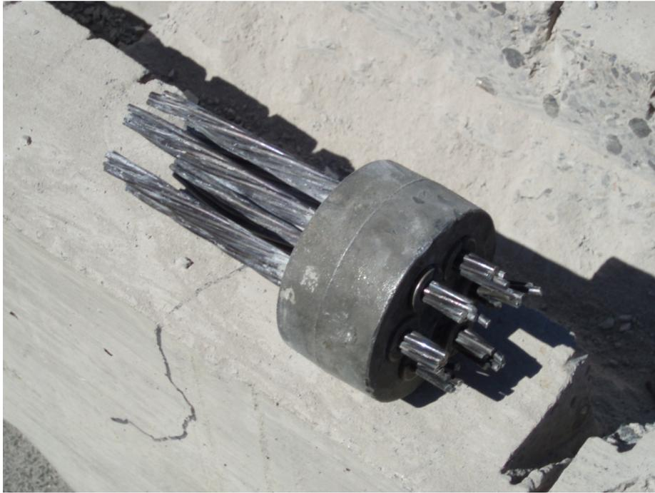
Figure H-6: Anchor Head and Strand After Removal from Anchorage
