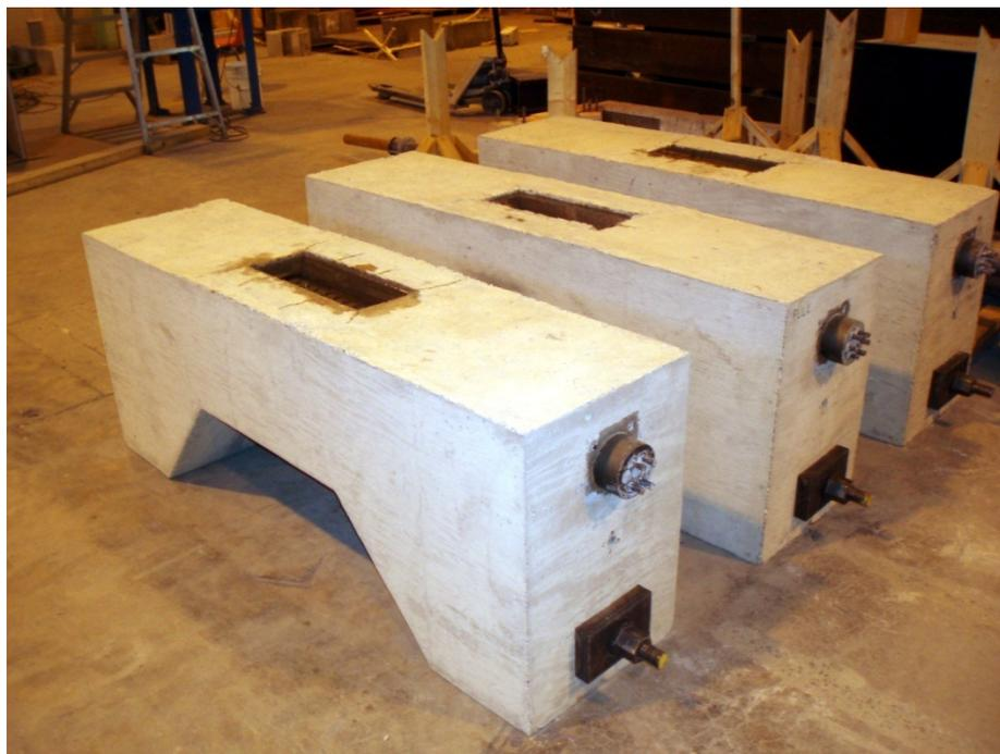
Figure C-9: Set of Three Specimens After Stressing of Post-Tensioning Bar
