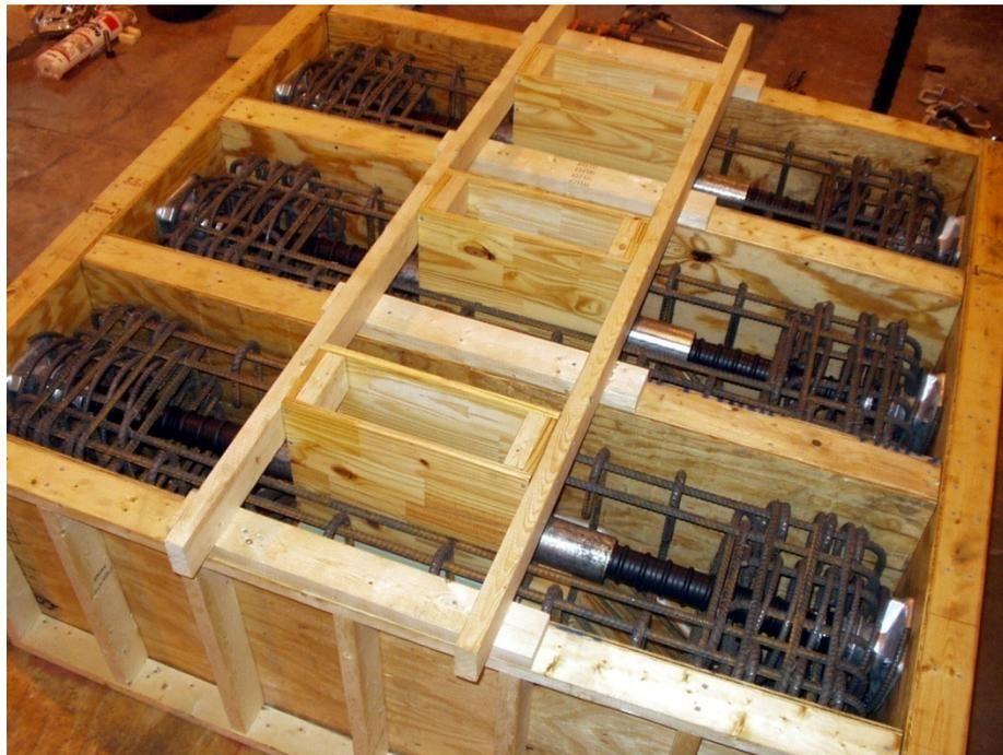
Figure 4-7: Completed Specimen Setup Ready for Concrete Placement
