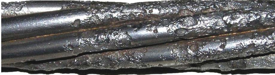
Figure A-2: Artificially Dense Pitting Structure
