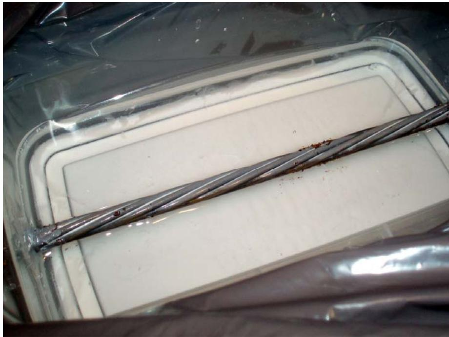
Figure 3-1: Non-Accelerated Corrosion Setup
