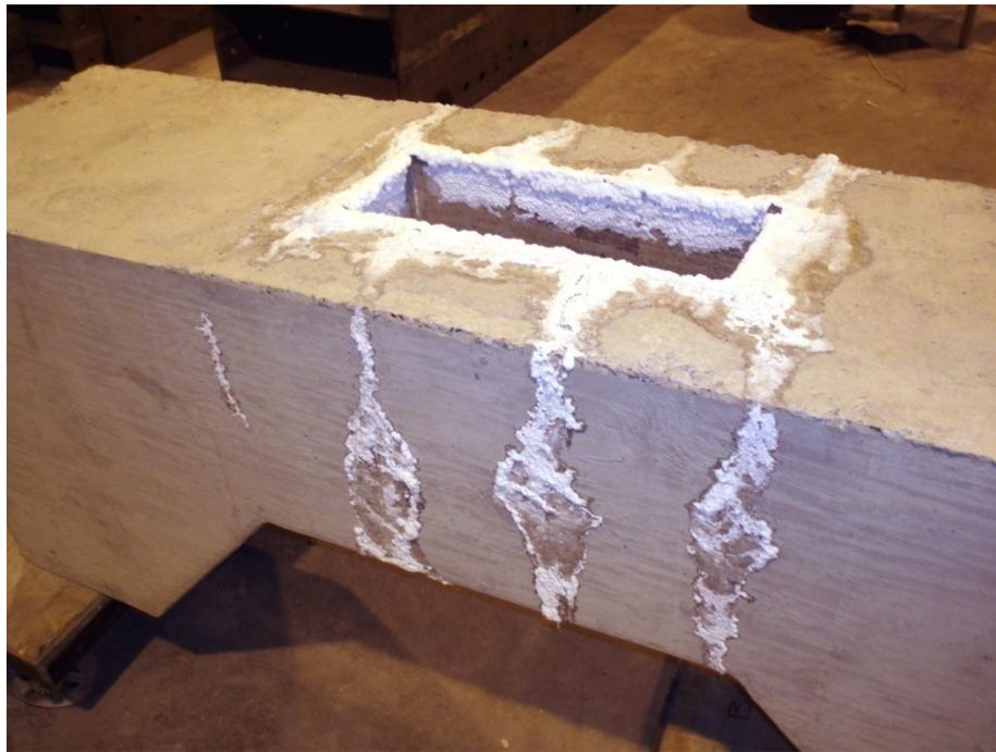
Figure 5-15: Beam Specimen GVC-2 After Six-Month Duration of Exposure Testing
