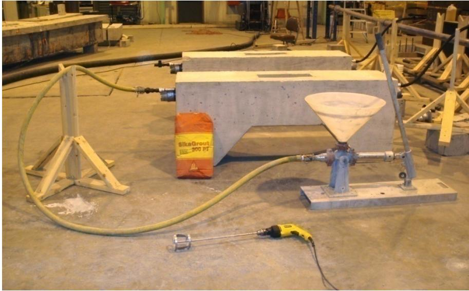
Figure C-6: Tendon Grouting Setup
