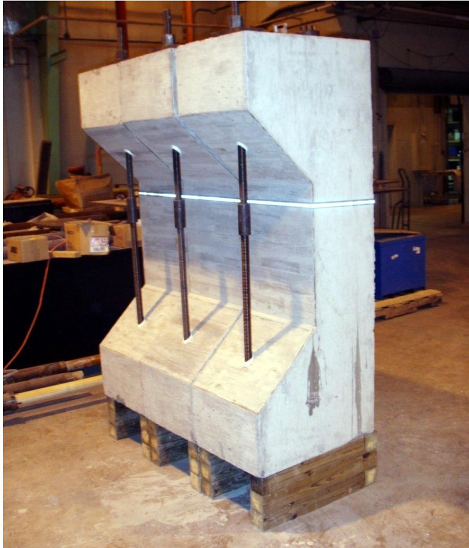
Figure 5-9: Anchor Zone Grout Void Corrosion Specimens Undergoing Exposure Testing
