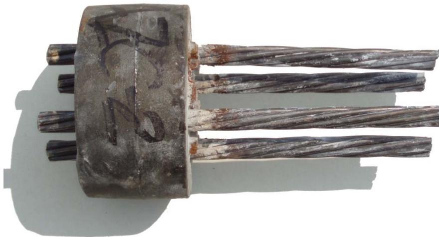
Figure 6-8: Strand Corrosion within Void Behind Anchor Head
