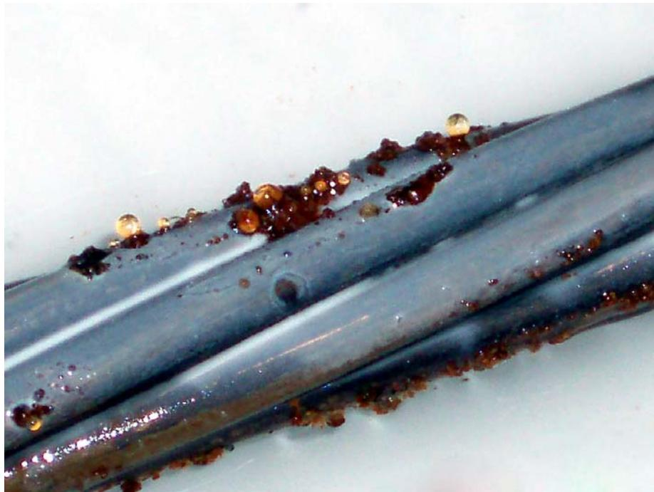
Figure 3-6: Hydrogen Evolution During Localized Corrosion Attack
