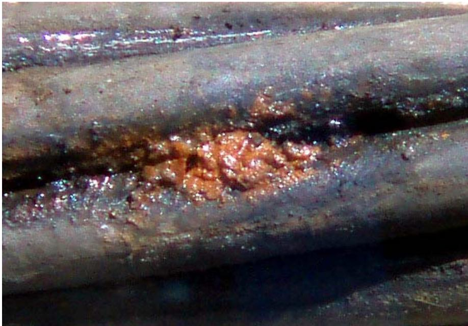
Figure 3-3: Crevice Corrosion Attack
