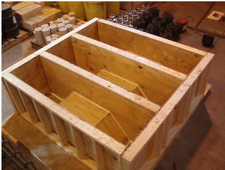
Figure C-1: Basic Formwork for Casting Specimens
