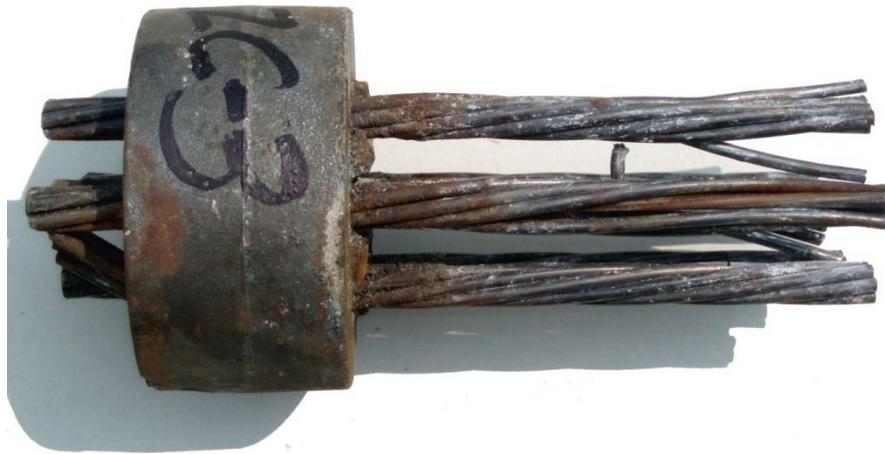
Figure 6-9: Strand Corrosion Within and Away from Grout Void
