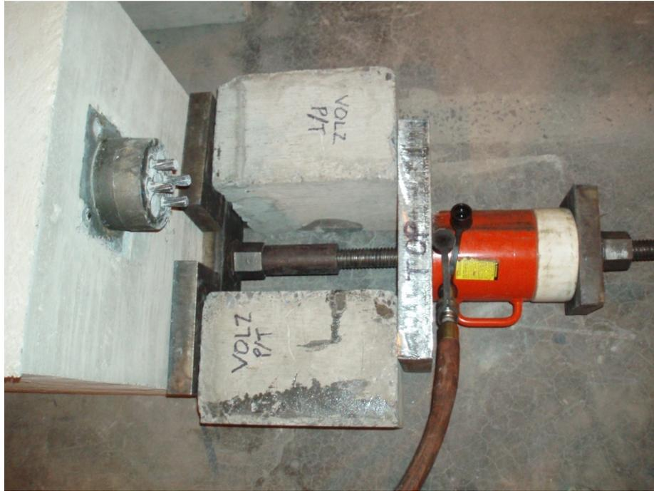
Figure C-8: Prestressing Bar Stressing Setup
