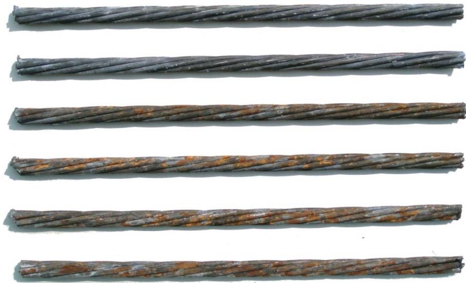
Figure 6-11: Strand Corrosion Experienced by GVC Beam Specimens
