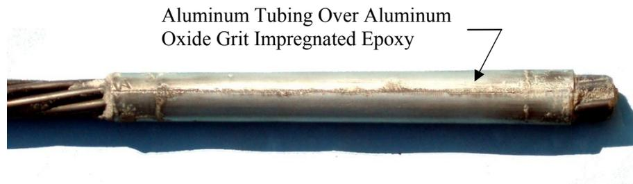
Figure 3-9: Strand Specimen End Treatment for Fatigue Testing
