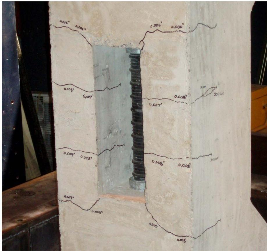
Figure 5-19: Typical Crack Pattern for Partially Prestressed Specimens
