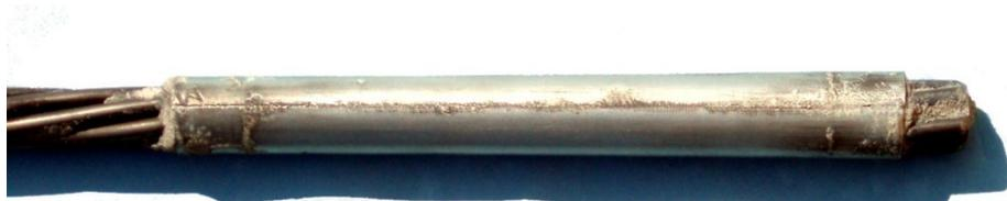
Figure B-1: Strand End Treatment for Fatigue Testing
