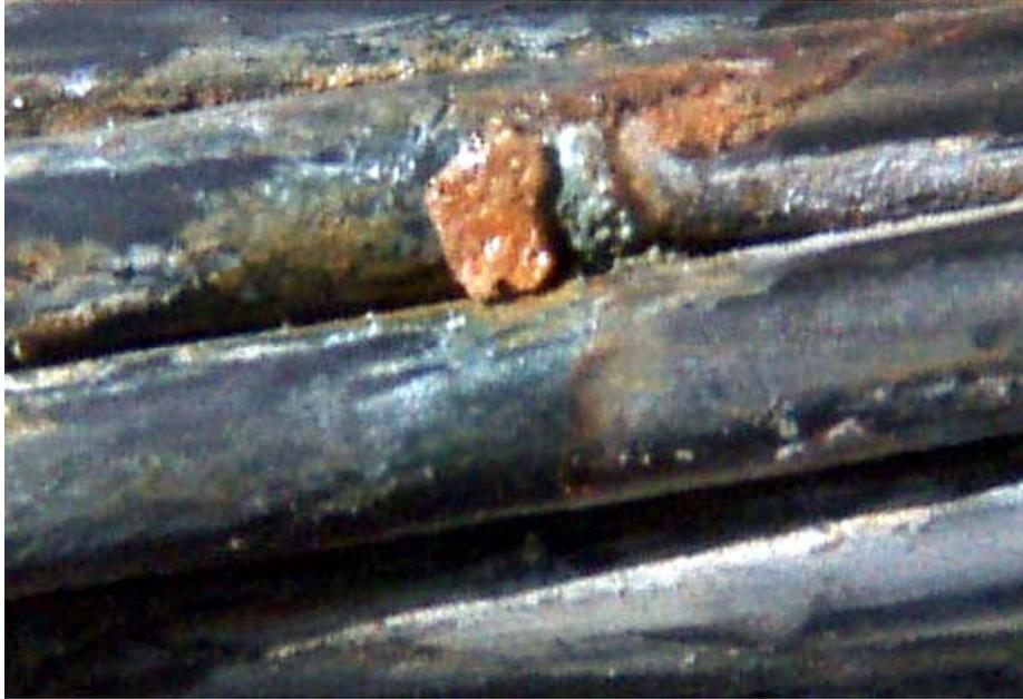
Figure 3-2: Pitting Corrosion Attack
