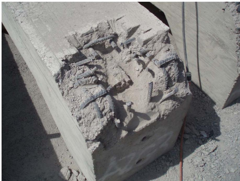
Figure H-5: Beam Specimen After Anchorage Removal
