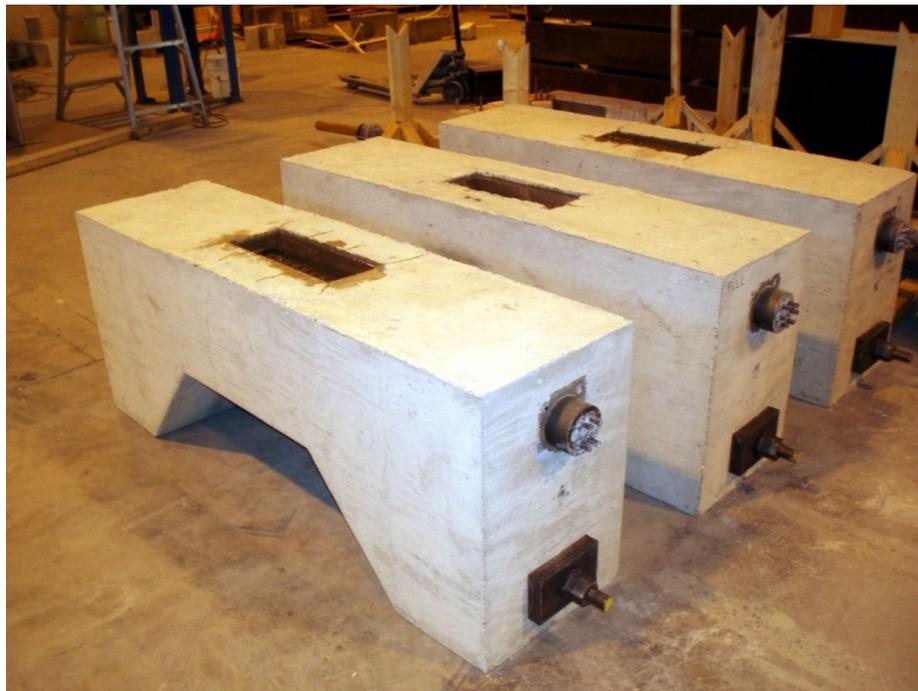
Figure 4-8: A Set of Three Completed Beam Specimens
