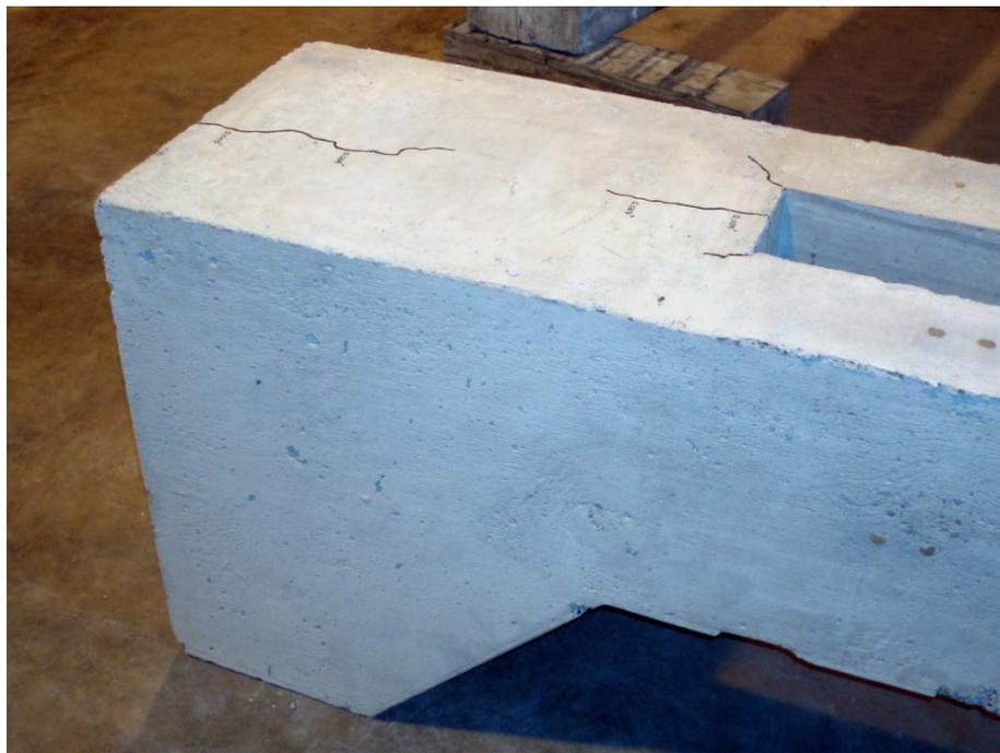
Figure F-3: Typical Longitudinal Cracking of Beam Specimens
