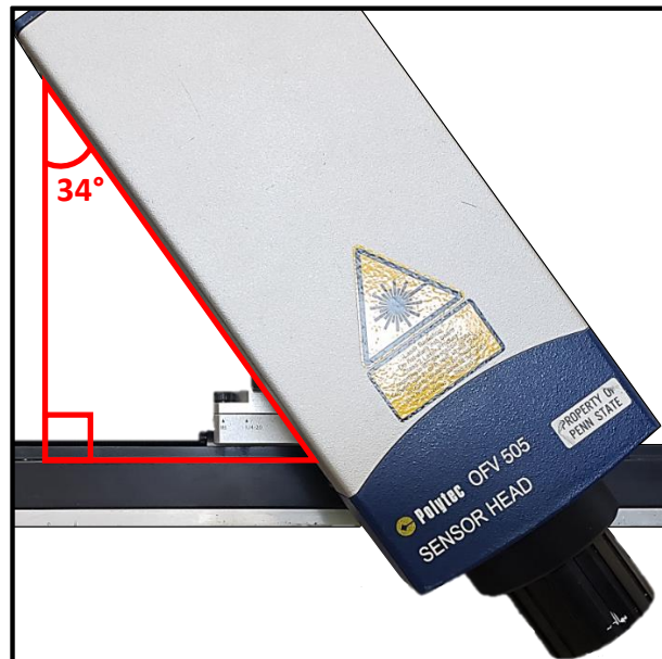
Figure 4-4: Laser Doppler Vibrometer (LDV) pointed at reflective tape in the transmitted region of the plate and angled 34^\circ from vertical to measure both in-plane and out-of-plane velocities
