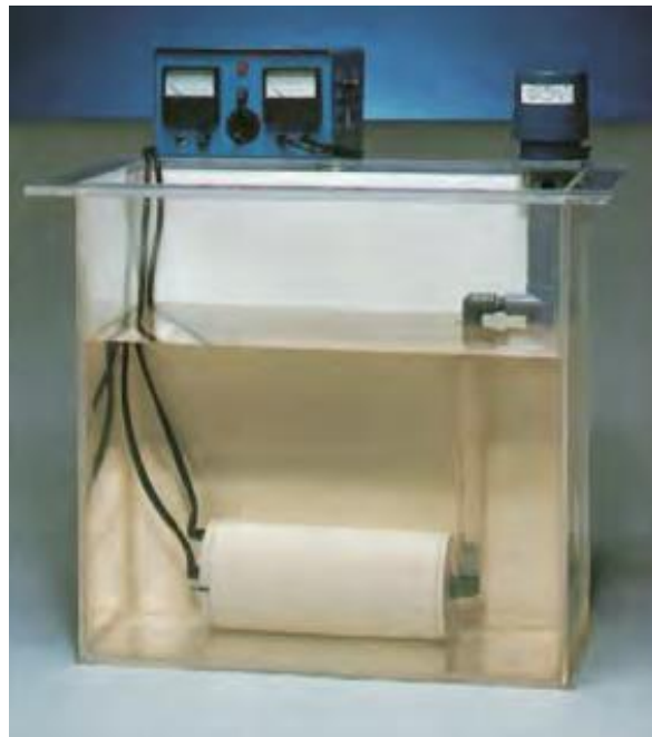
Figure 9. Copper Electrowinning System (PMPC, 2017)
