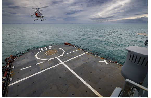
(b) Airbus tests VSR700 autonomous landing system using optionally piloted aircraft (from [4]).
