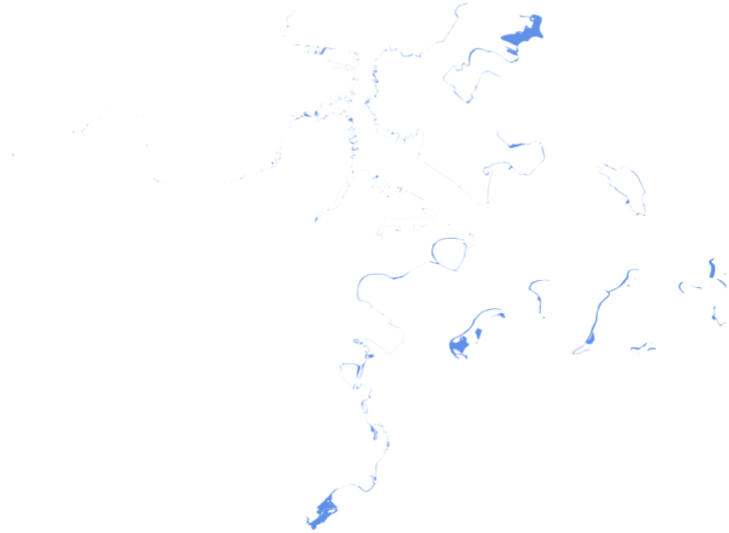
Figure 3-2: 2030 (9-inch increase) SLR shapefile projection of Boston after being clipped to the Boston boundary shapefile. Blue areas show locations that are not currently underwater but are projected to be in 2030.
