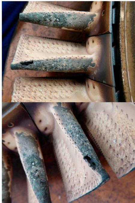
Figure 1-1. Burned through high pressure turbine blade. Image from [4]
