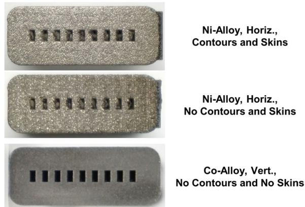
**Figure 7-4. Pictures of several as-built test coupons.**
