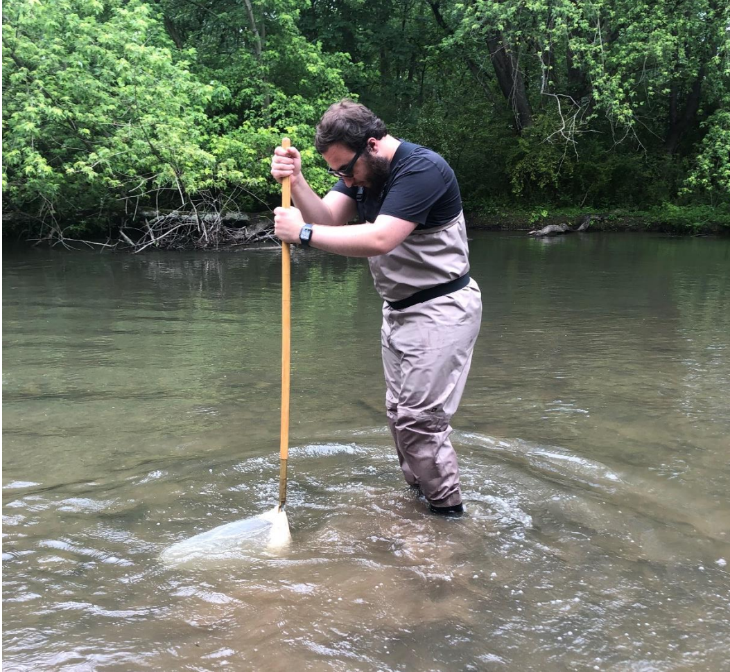
Figure 9. D frame kick net sampling for macroinvertebrates in the Shenango River at the Halfway Road Bridge
