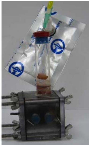
Figure 3.4 Setup for the GBM, the cell is attached directly to a gas bag.
