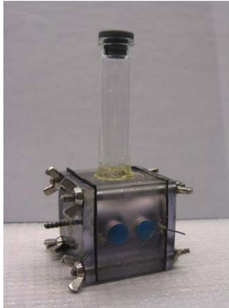
Figure 3.2: Picture of a typical MEC cell with brush anode on left and cathode (either platinum or SS304 mesh) on right [49]
