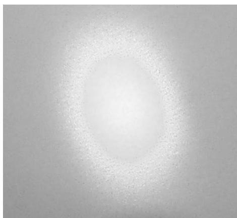
Figure 3.19: Output laser spatial profile after exiting from the NLC waveguide.
