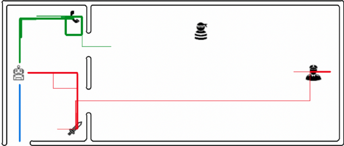
Figure 4.7: Pathlines of execution policies during testing. Each policy was tested graphically five times to generate the paths shown. Blue represents the paths for \pi_{hide}^E , green for \pi_{call}^E and red for \pi_{kill}^E .
