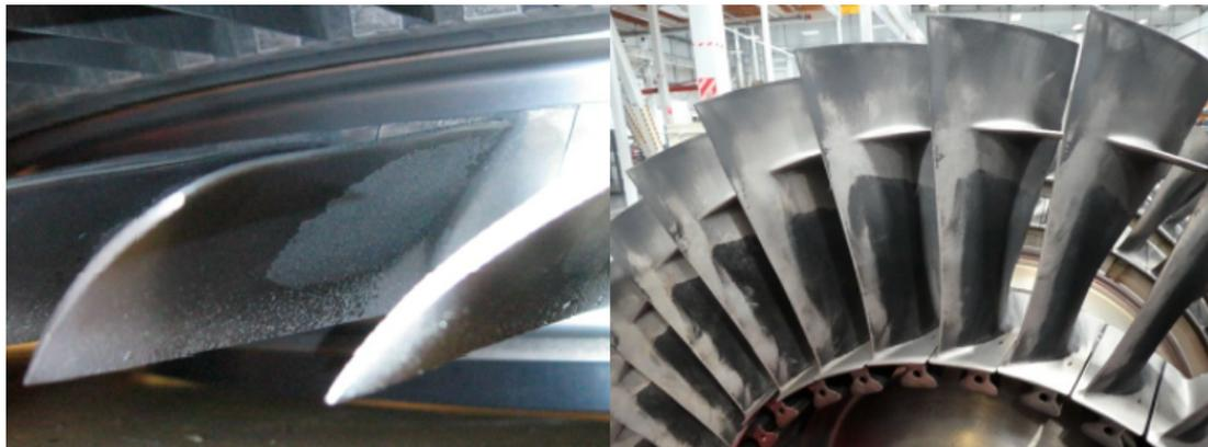
**Figure 6.1.** Different examples of deposition of particulate matter on axial compressor blades [12]
