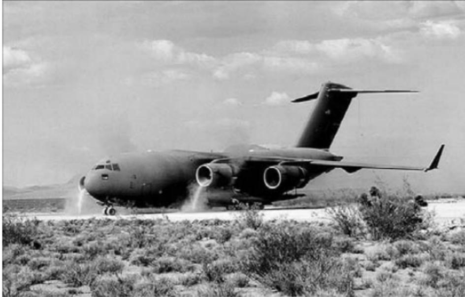
**Figure 1.2.** A view of sand being ingested into a C-17 at take-off [9]
