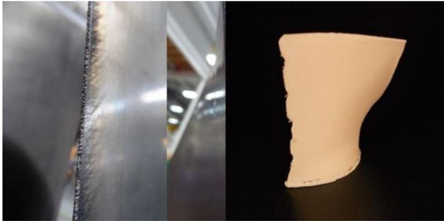
**Figure 2.5.** Original [12] and 3D printed blades with Cragged damage
