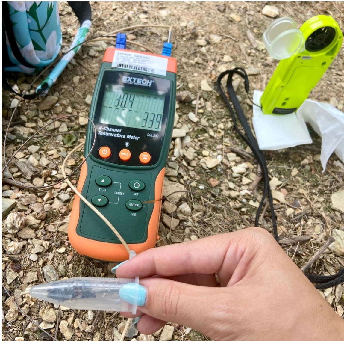
Figure 4-3: Kestrel (5500AG Agriculture Weather Meter) and thermocouple thermometer (RTD/Thermocouple (SDL200-Nist)) paired with the flat probe and the stab probe thermocouples at Vynecrest Winery in Breinigsville, PA.
