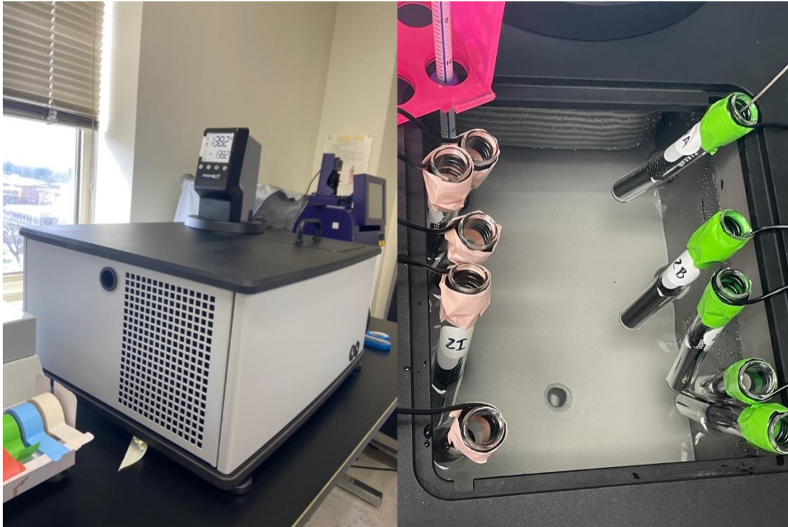
Figure 3-2: Circulating water bath (VWR- 7L low profile, refrigerated circulator with MX controller containing a mix of ethylene glycol and water in equal amounts) used for CTmin, LLT, and LLt (Left). Ten lab-reared first instar SLF nymphs submerged into bath in 13mm x 100mm Pyrex glass test tube, with one thermocouple (Type K) for CTmin (Right).
