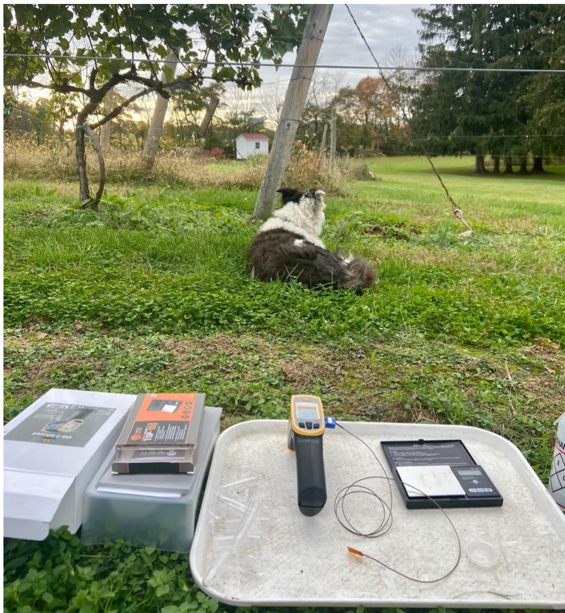
Figure 4-1: Scale and infrared thermometer (Industrial IR with Circle Laser (IRK-2)) and a thermocouple (Type K) attached, fitted with a 0.38 inch by 1.0-inch flat elongated probe at Private Growers in Coopersburg, PA.
