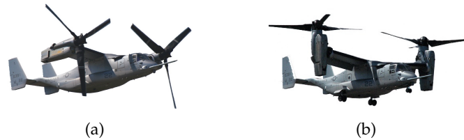
Figure 3.12: Depiction of the rotation of the Osprey's nacelles to achieve airplane and helicopter configurations [18, 19].
