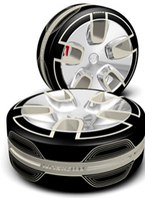
Figure 3.6: Michelin's E.A.P. concept tires that can change tread pattern and depth for varying road conditions [10].
