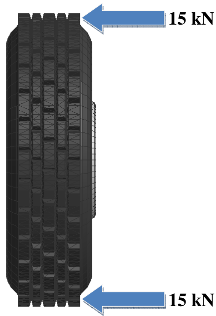
Figure 6.1: Out-of-plane translational excitation of the sidewall.
