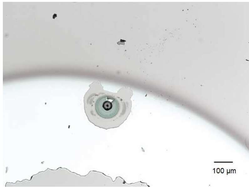
Optical image showing dielectric breakdown event not included in Fig 4.22
