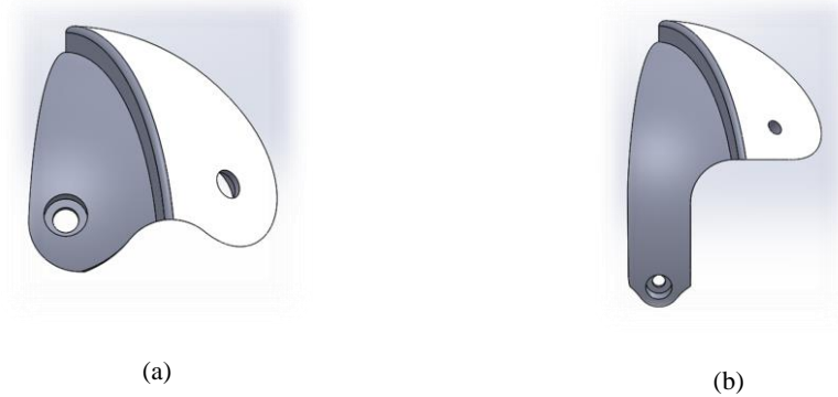
Figure 5-8: Blade design (a) first design (b) second design
