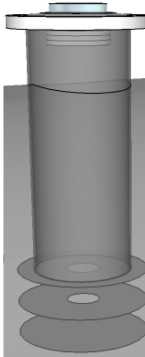
Figure 3.8 Schematic of the velocity map imaging setup. From bottom to top: the repeller electrode, the grounded electrode, the extractor electrode mounted on the flight tube, the microchannel plate and phosphor screen stack, the end flange, and the window.
