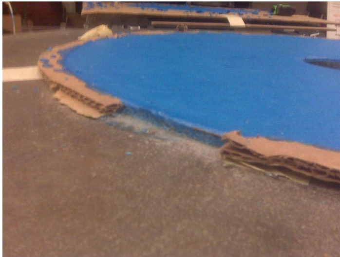
Figure 3-3: Photograph of Nansulate EPX Applied to Top Plate
