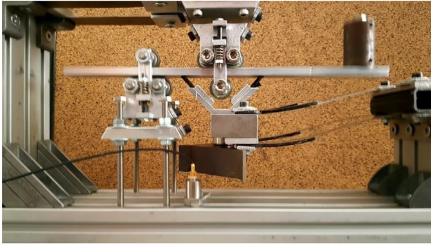
Figure 1.2. Schematic of a dynamic antiresonant vibration isolator.
