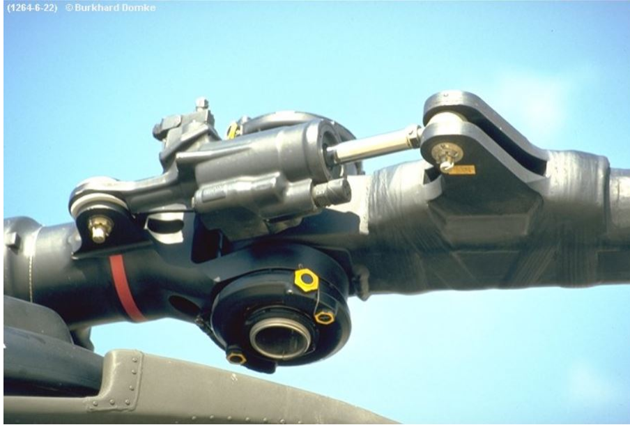
Figure 1.6. Fluidlastic Technology used on the rotor hub of CH-47 Chinook helicopter [5]
