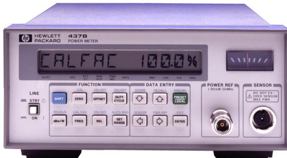
**Figure 2.8:** Hewlett Packard 437B power meter, used to convert the received analog signal into a digital form. Measured either in watts or dBm.
