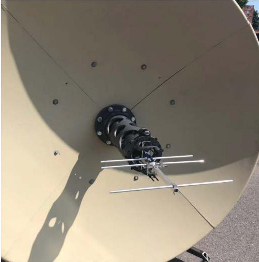
**Figure 2.1:** The 2.4 meter parabolic reflector used in conjunction with the 3-element Yagi-Uda antenna. Also known as a radio telescope.
