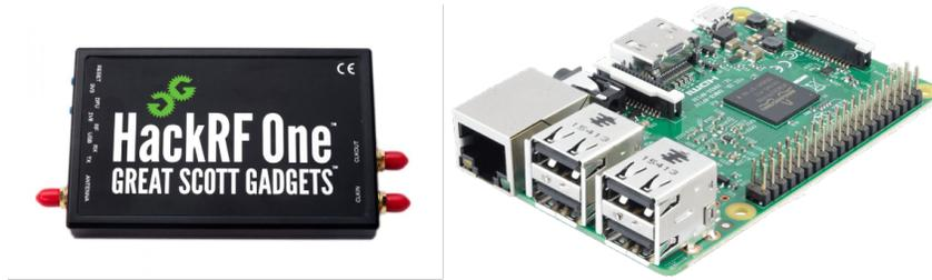
**Figure 4.5:** The HackRF One SDR. Very versatile with a half-plex setup. Used to filter and measure the signal collected by the radio-telescope.
