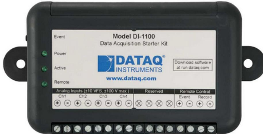
**Figure 2.9:** Data Acquisition Device, used to measure signal from the power meter, along with recording and storing the data.
