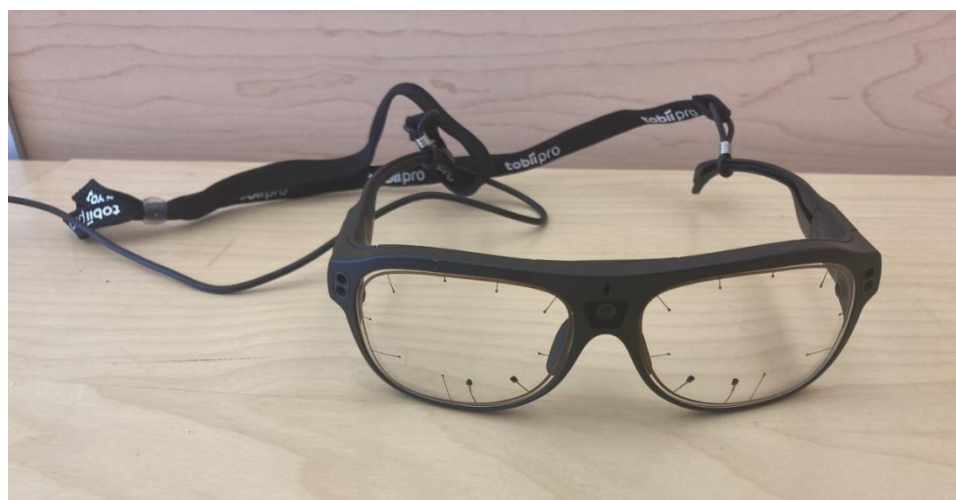
Figure 2-1: Tobii glasses showing front facing camera and infrared sensors in the lenses
