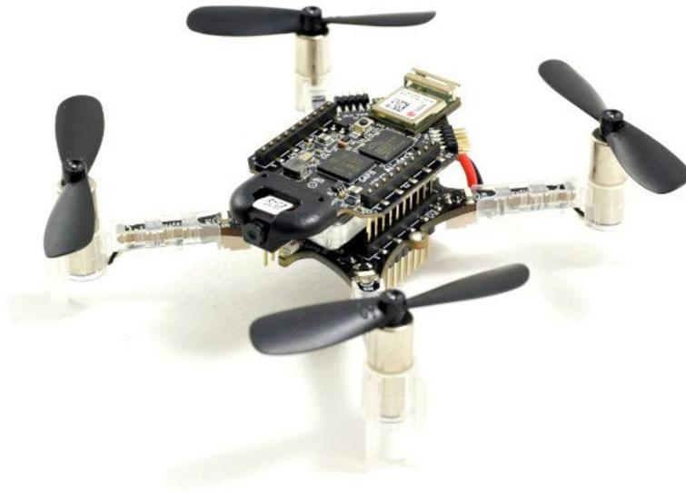
**Figure 1.2.** The Crazyflie 2.1 with AI Deck attached.
